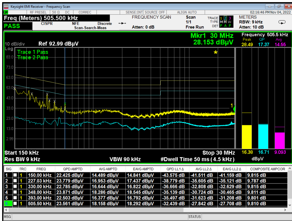
Figure 12 - Conducted Emissions Plot, Neutral, IDLE
