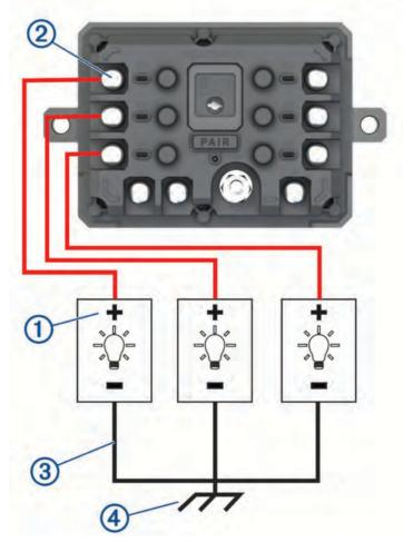
2 Connect the negative or ground wire ③ to an unpainted ground stud ④ on the vehicle frame, to a ground distribution block, or directly to the negative terminal on the battery.
