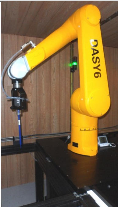
DASY 6 SAR System with SAM Phantom
