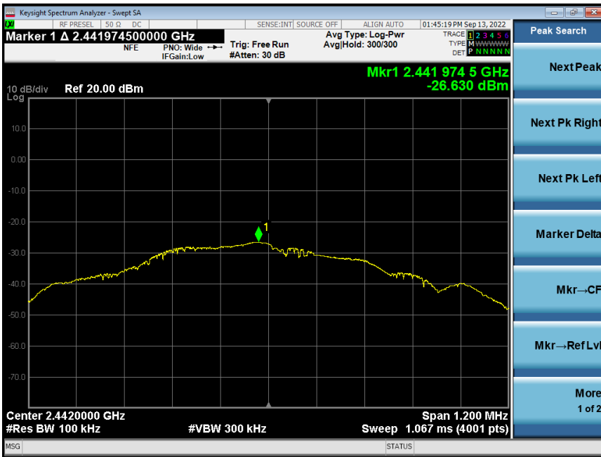
Figure Tr17.5: Partially corrected power spectral density data for ANT, 2442 MHz
