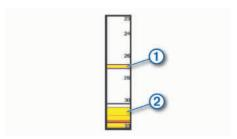
The a-scope above shows fish returns  $\bigcirc$  and a soft bottom return  $\bigcirc$ .
