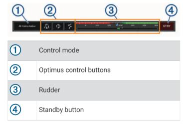
You must press a mode button on the overlay bar to engage or disengage the mode. When the mode is engaged, the button is illuminated.
