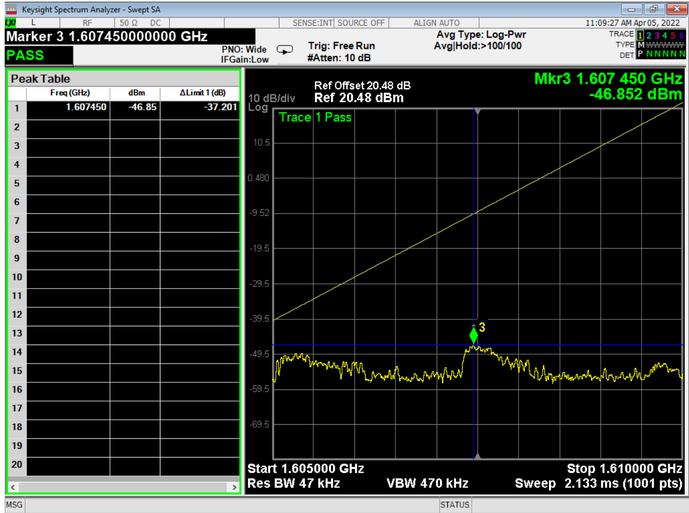
Figure 12 – Part 25.216(g), Transmitting at 1620.979126 MHz, Conducted Measurement *Limits have been converted from dBW to dBm. dBW = dBm + 30
