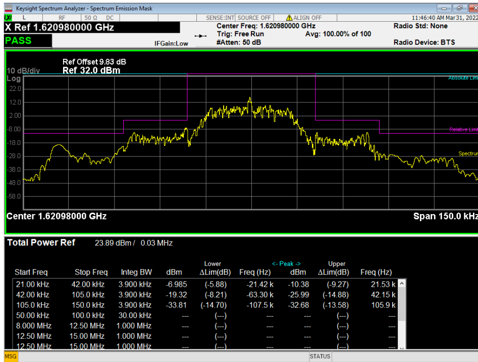
Figure 6 – Part 25.202(f) Mask, Transmitting at 1620.979126 MHz
