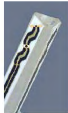
Figure 2.3 Probe Thick-Film Technique
