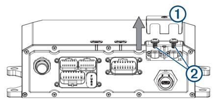
2 Remove the screws from the GND terminal and the +12V terminal 2.
