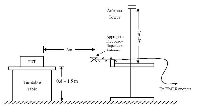
Diagram 2 Test arrangement for radiated emissions tested on Open Area Test Site (OATS)
