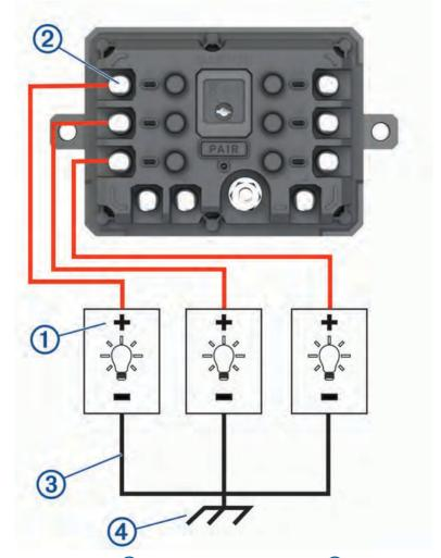
2 Connect the negative or ground wire ③ to an unpainted ground stud ④ on the vehicle frame, to a ground distribution block, or directly to the negative terminal on the battery.
