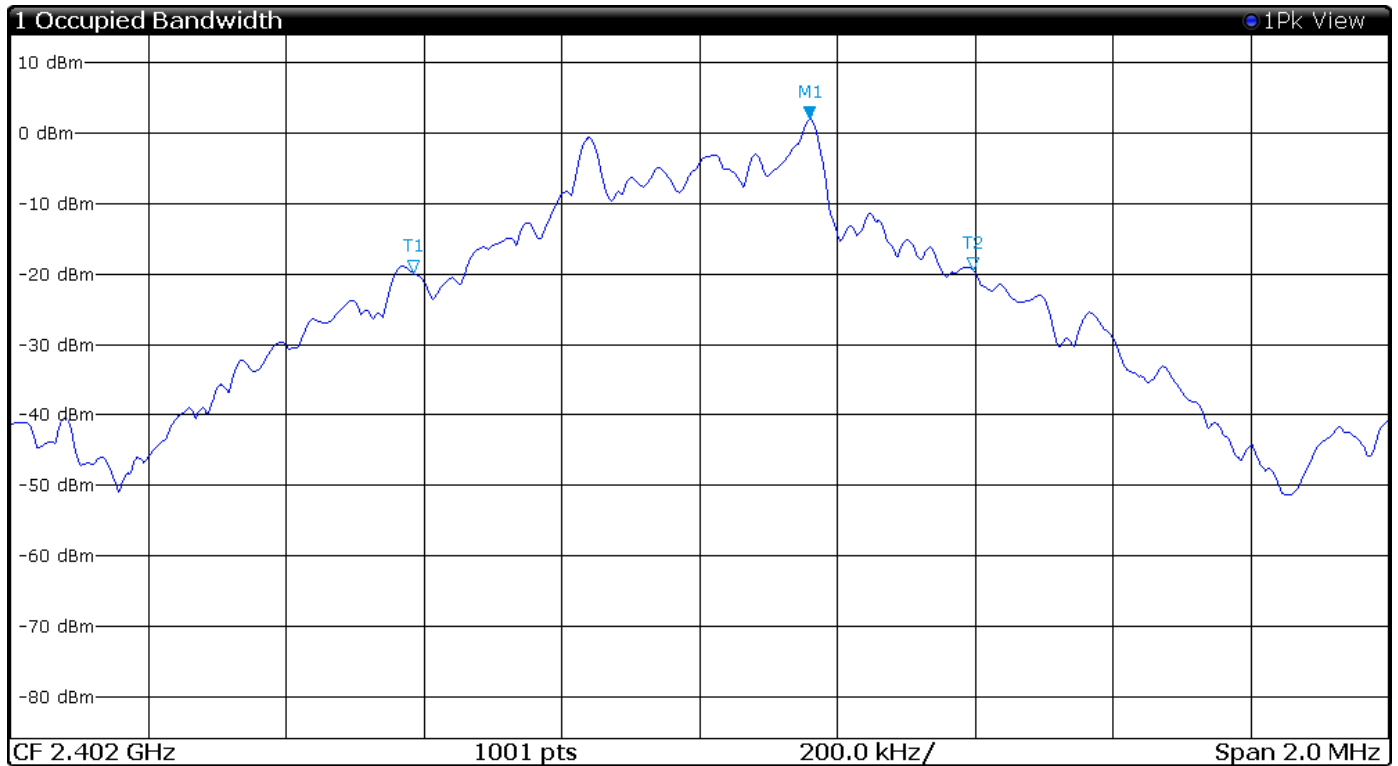
Figure 7 Plot of Transmitter Emissions 99% Occupied Bandwidth Mode 1 BT BR
