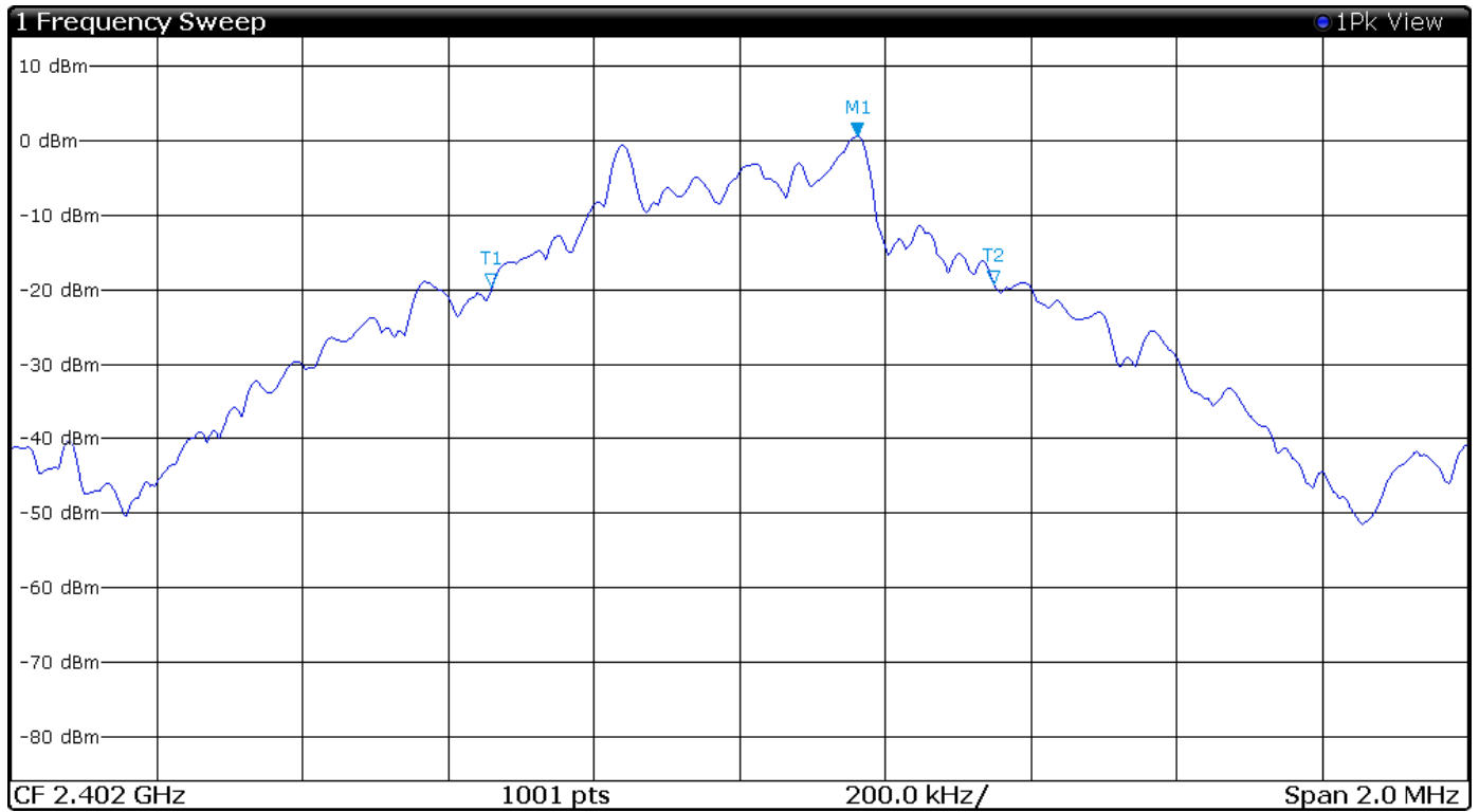
Figure 6 Plot of Transmitter Emissions 20-dB Occupied Bandwidth Mode 1 BT BR
