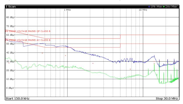
Figure 4 AC Line Conducted emissions of EUT line 2 (EUT – Computer)
