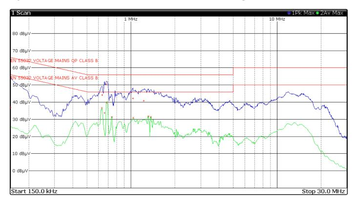
Figure 2 AC Line Conducted emissions of EUT line 2 (EUT – AC Adapter)
