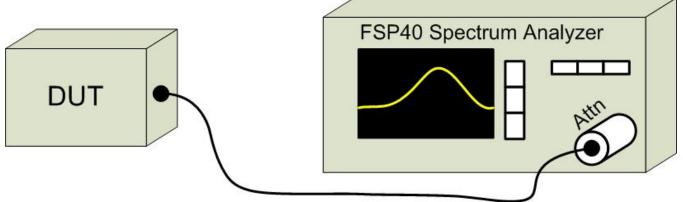
Figure A.1 – Test Setup Conducted Measurements
