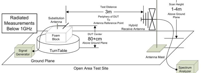
Figure A.4 – Test Setup Radiated Emissions Measurements 30 – 1000MHz Signal Substitution
