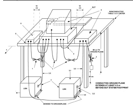
Figure A.7 – Test Setup Conducted Emissions Measurements
