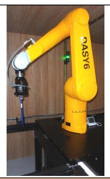
**DASY 6 SAR System with SAM Phantom**
