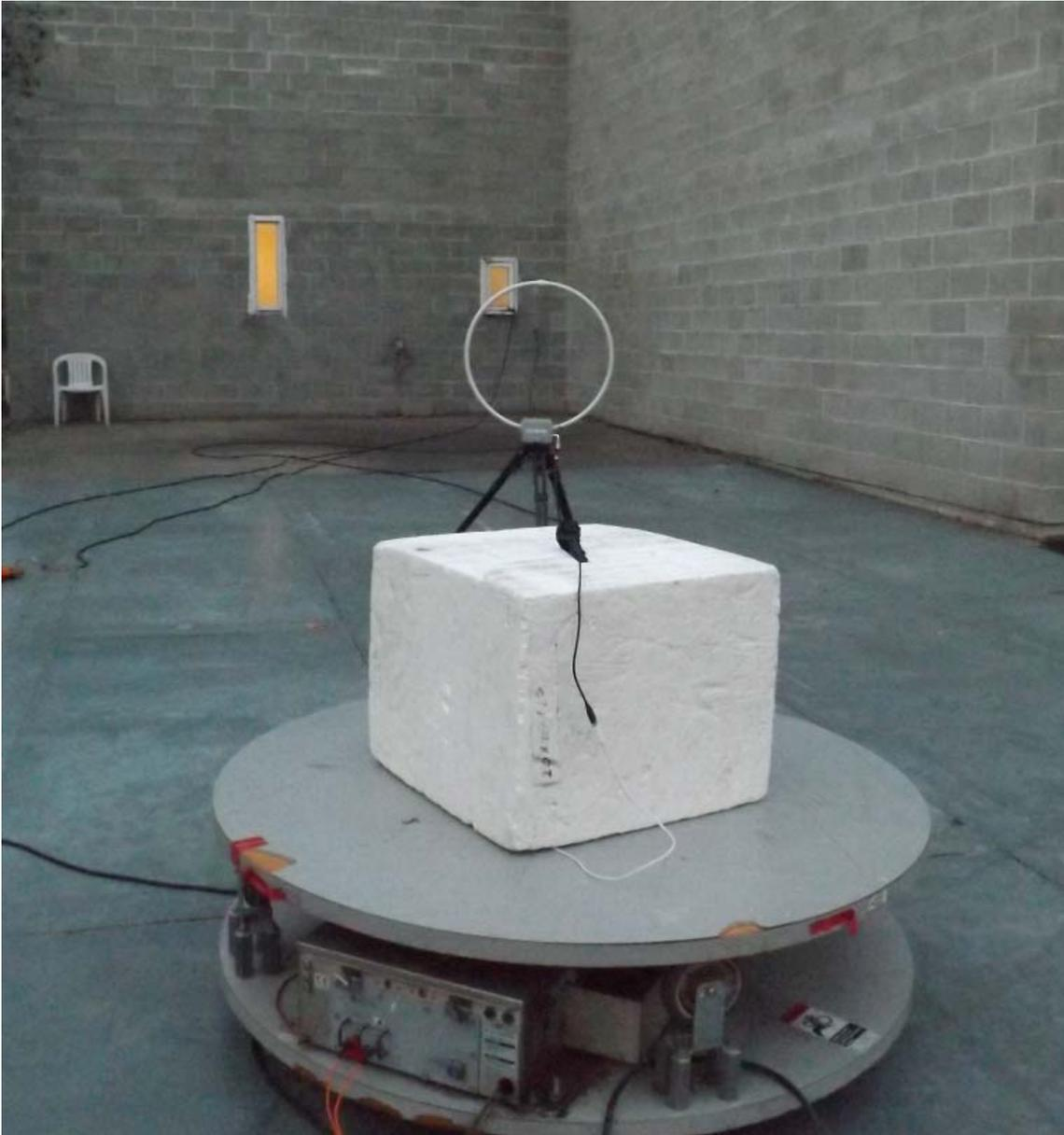
**Figure E20.2 – Setup Photo – Radiated Measurements 30 - 1000MHz**
