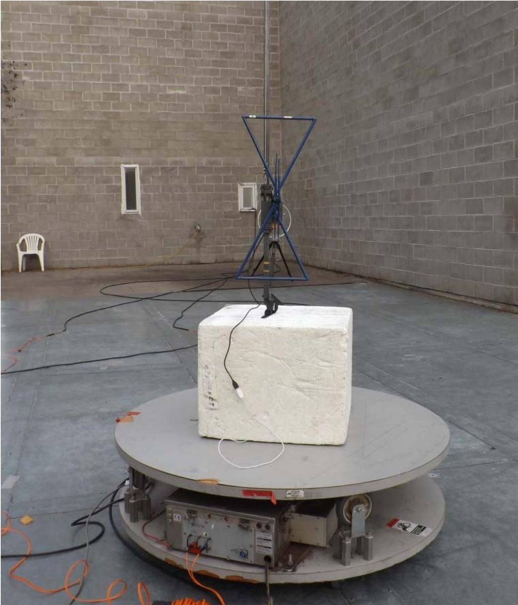
**Figure E20.3 – Setup Photo – Radiated Measurements 1 – 18GHz**
