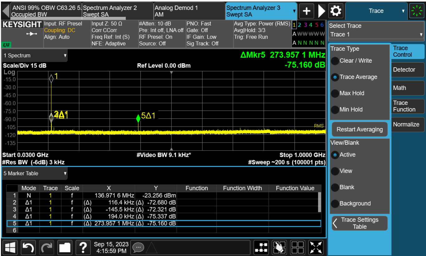
Figure TR4.6: Spurious emission graphical data for 136.975 MHz, 16W
