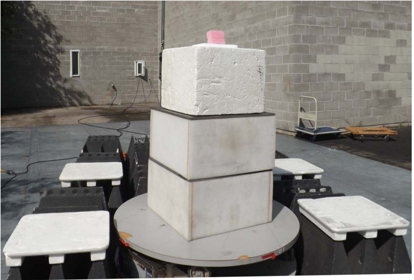
Figure E20.9 – Setup Photo – Radiated Measurements – 18-25GHz, Vertical
