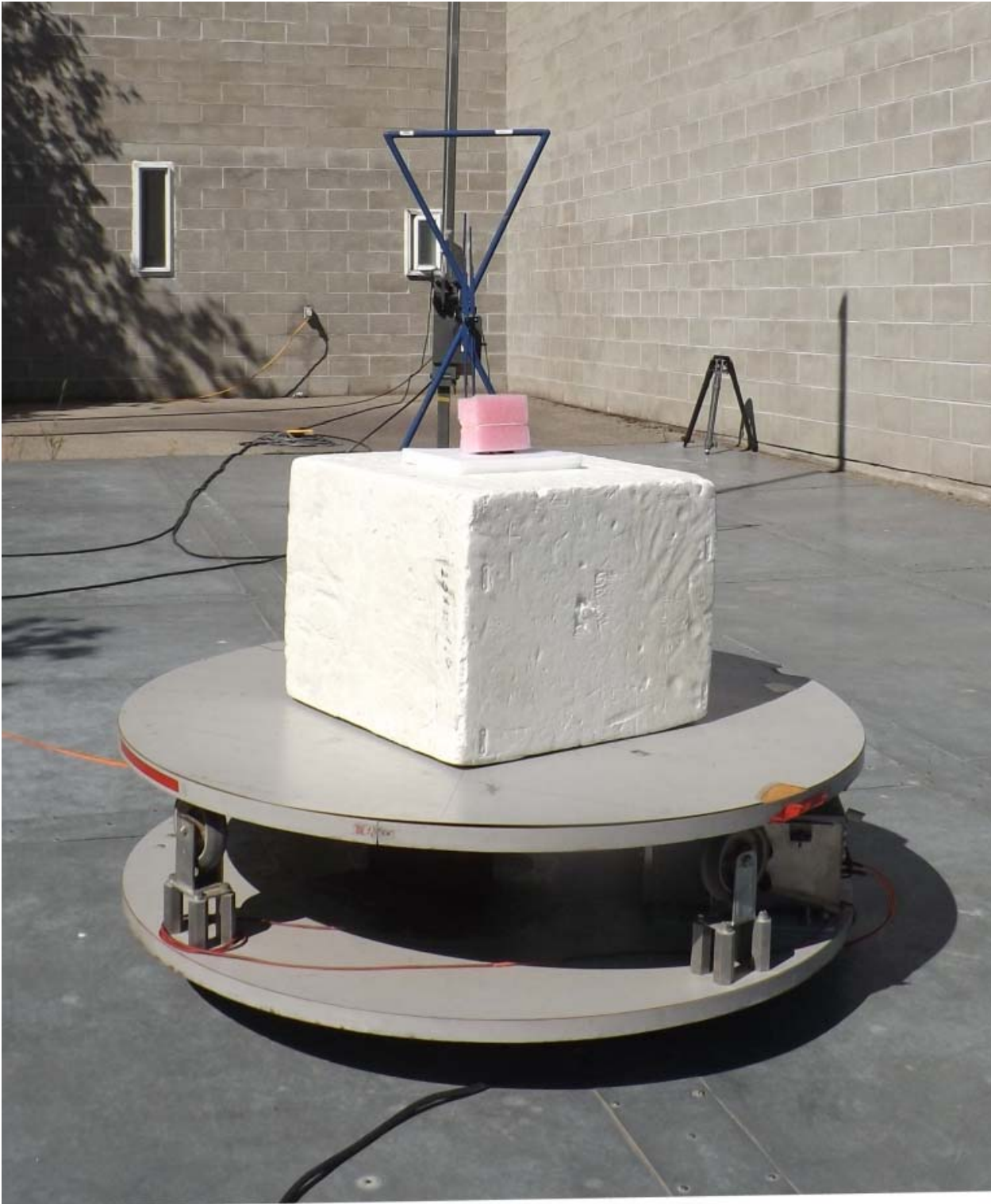
Figure E20.3 – Setup Photo – Radiated Measurements – 30-1000MHz, Vertical
