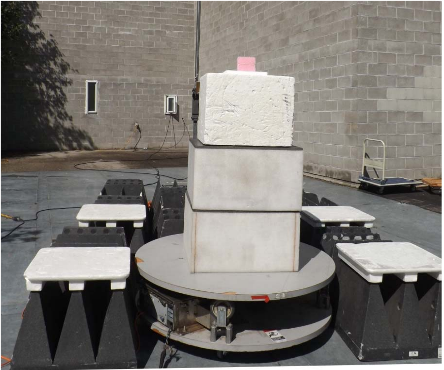
Figure E20.7 – Setup Photo – Radiated Measurements – 1-18GHz, Vertical
