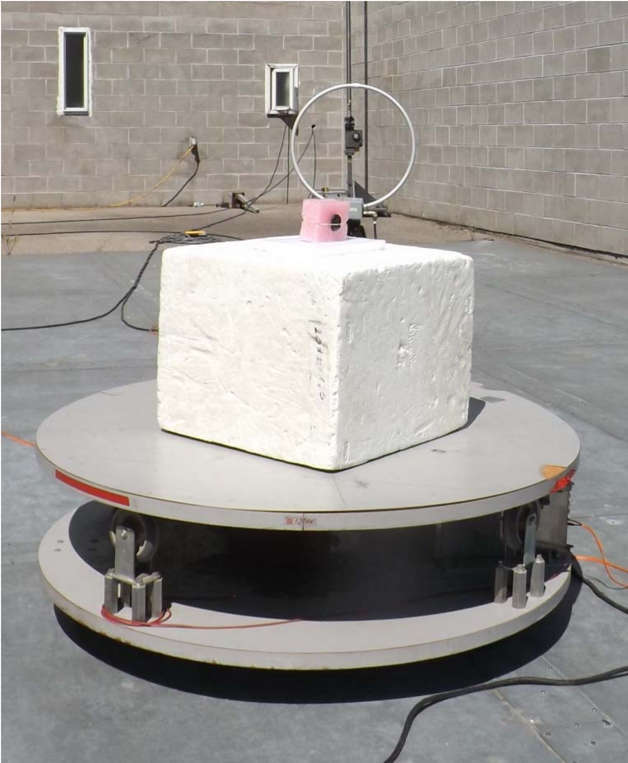
Figure E20.4 – Setup Photo – Radiated Measurements – Below 30 MHz, Front
