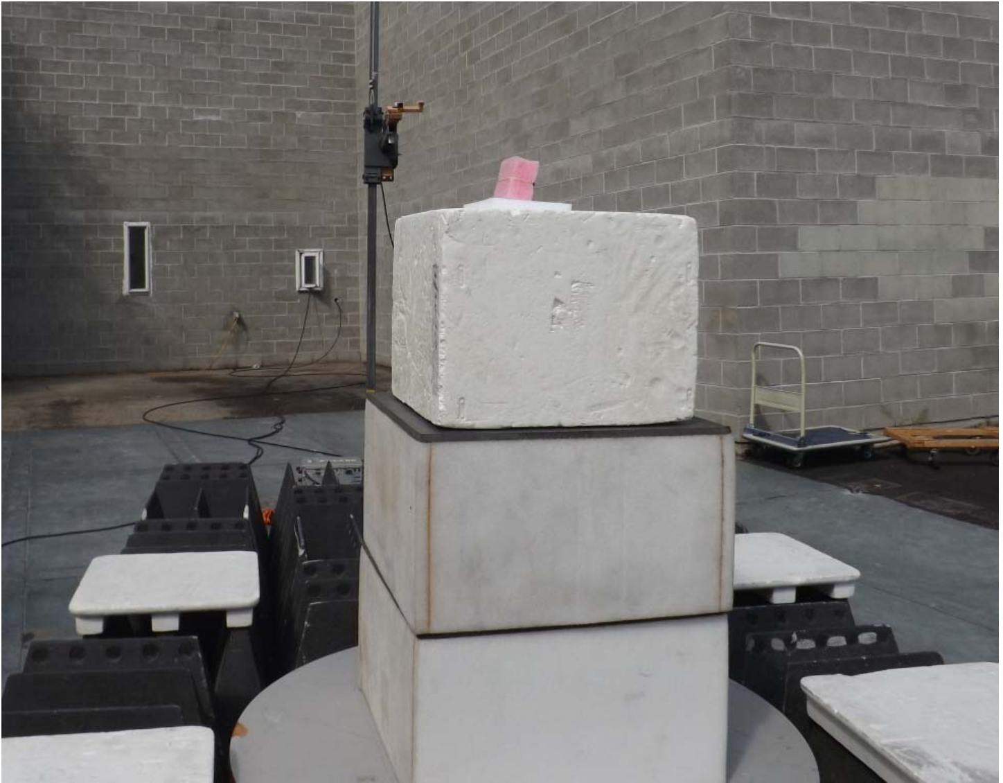
Figure E20.8 – Setup Photo – Radiated Measurements – 18-25GHz, Horizontal
