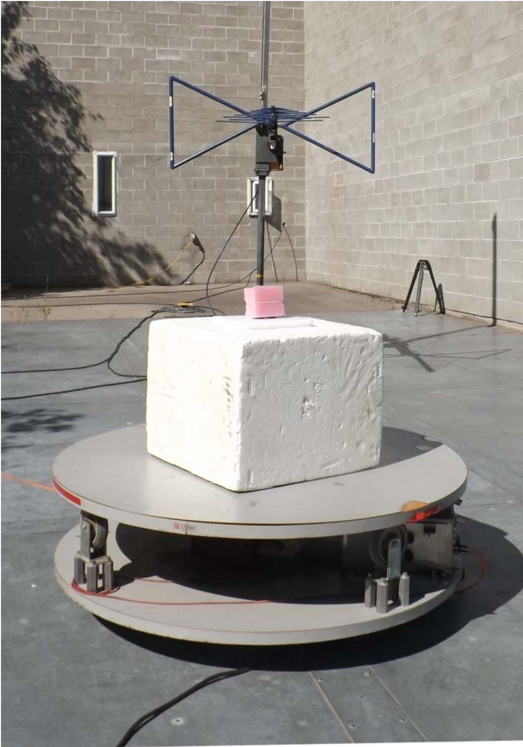
Figure E20.2 – Setup Photo – Radiated Measurements – 30-1000MHz, Horizontal
