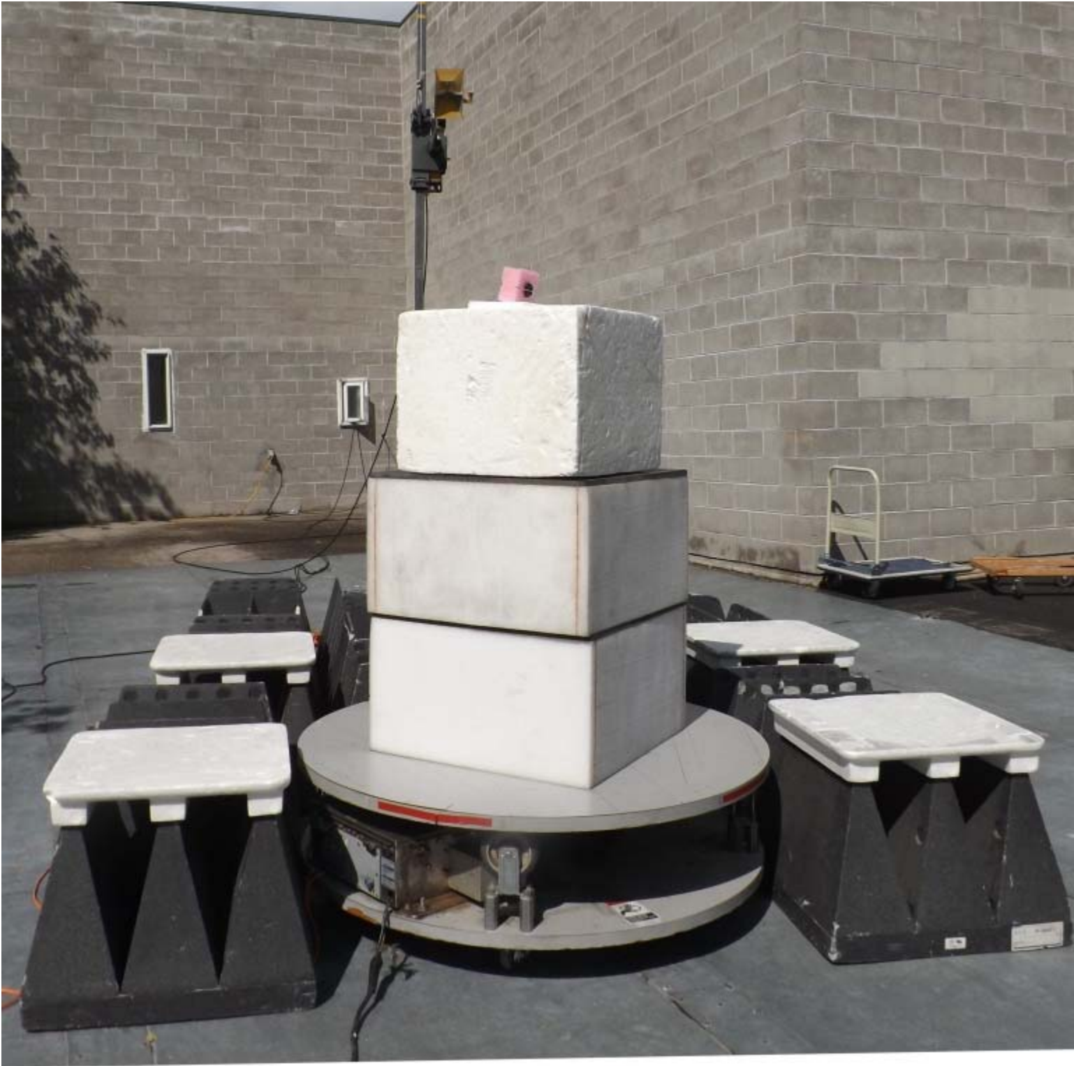
Figure E20.6 – Setup Photo – Radiated Measurements – 1-18GHz, Horizontal
