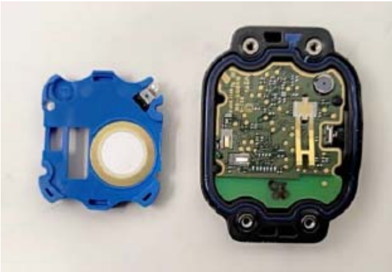
Figure E19.2 – Internal Photo –Cover / PCB
