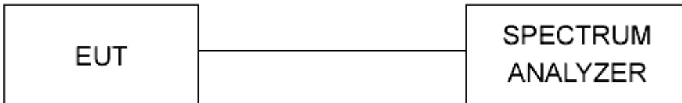
Figure 7 - Bandwidth Measurements Test Setup
