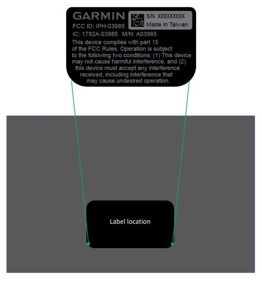
The label is screen-printed on vinyl material and is intended to be permanent and last the lifetime of the device.
