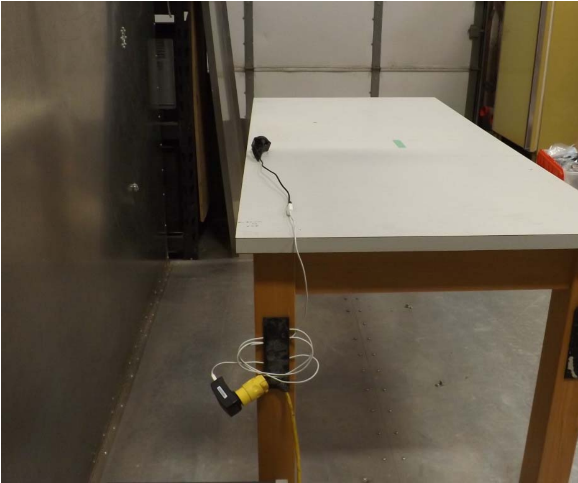
Figure E20.8 – Setup Photo – Power Line Conducted Emissions
