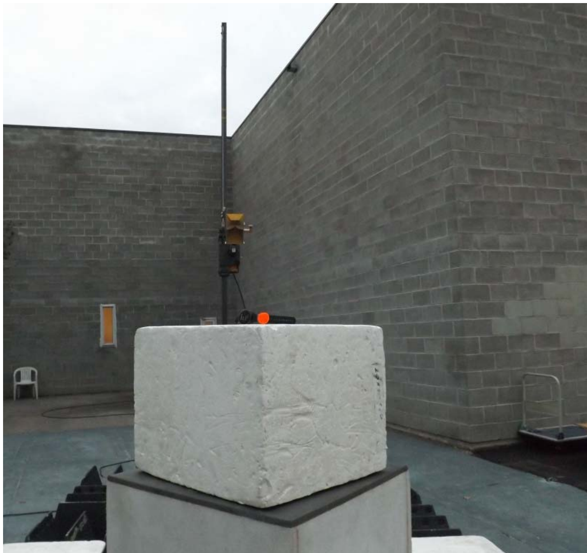
Figure E20.4 – Setup Photo – Radiated Measurements 1 – 18GHz
