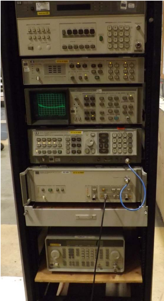
Figure E20.9 – Setup Photo – Power Line Conducted Emissions
