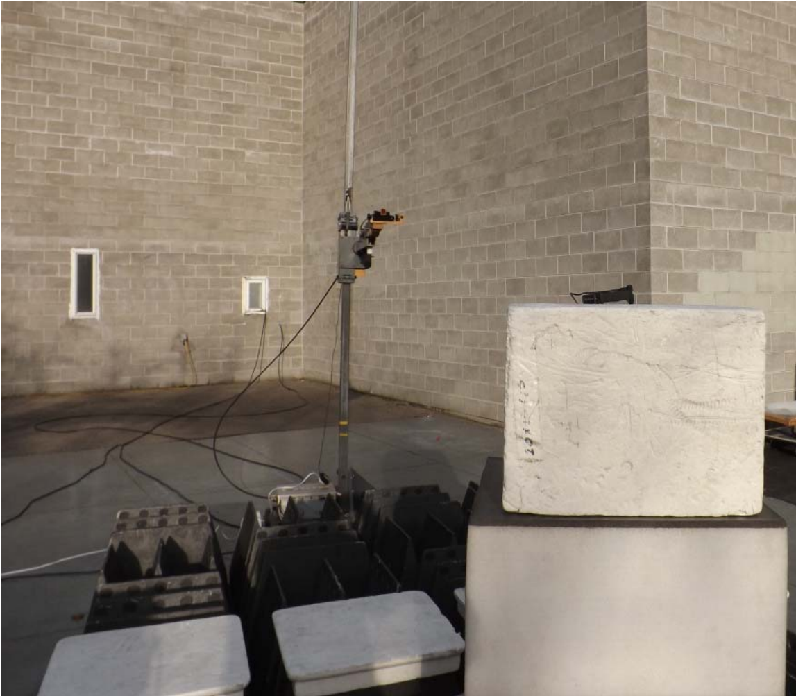
Figure E20.5 – Setup Photo – Radiated Measurements 18 – 26GHz
