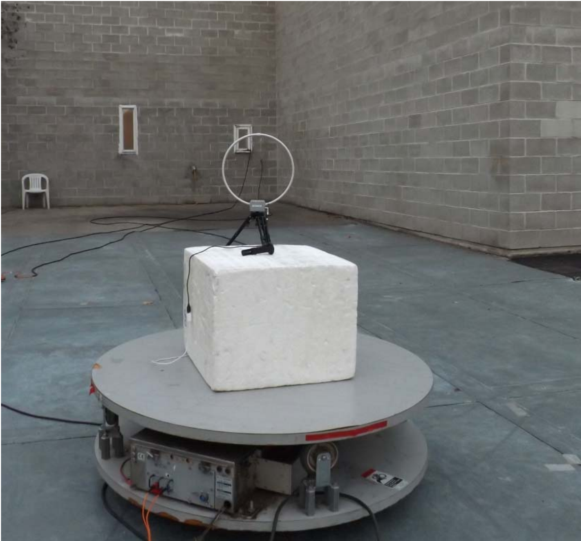
Figure E20.2 – Setup Photo – Radiated Measurements 9kHz – 30MHz
