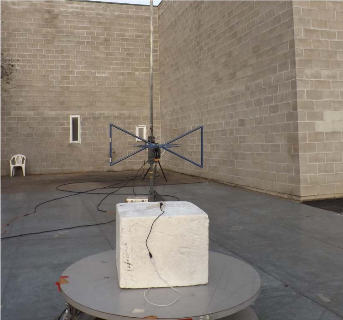
**Figure E20.4 – Setup Photo – Radiated Measurements 1 – 18GHz**
