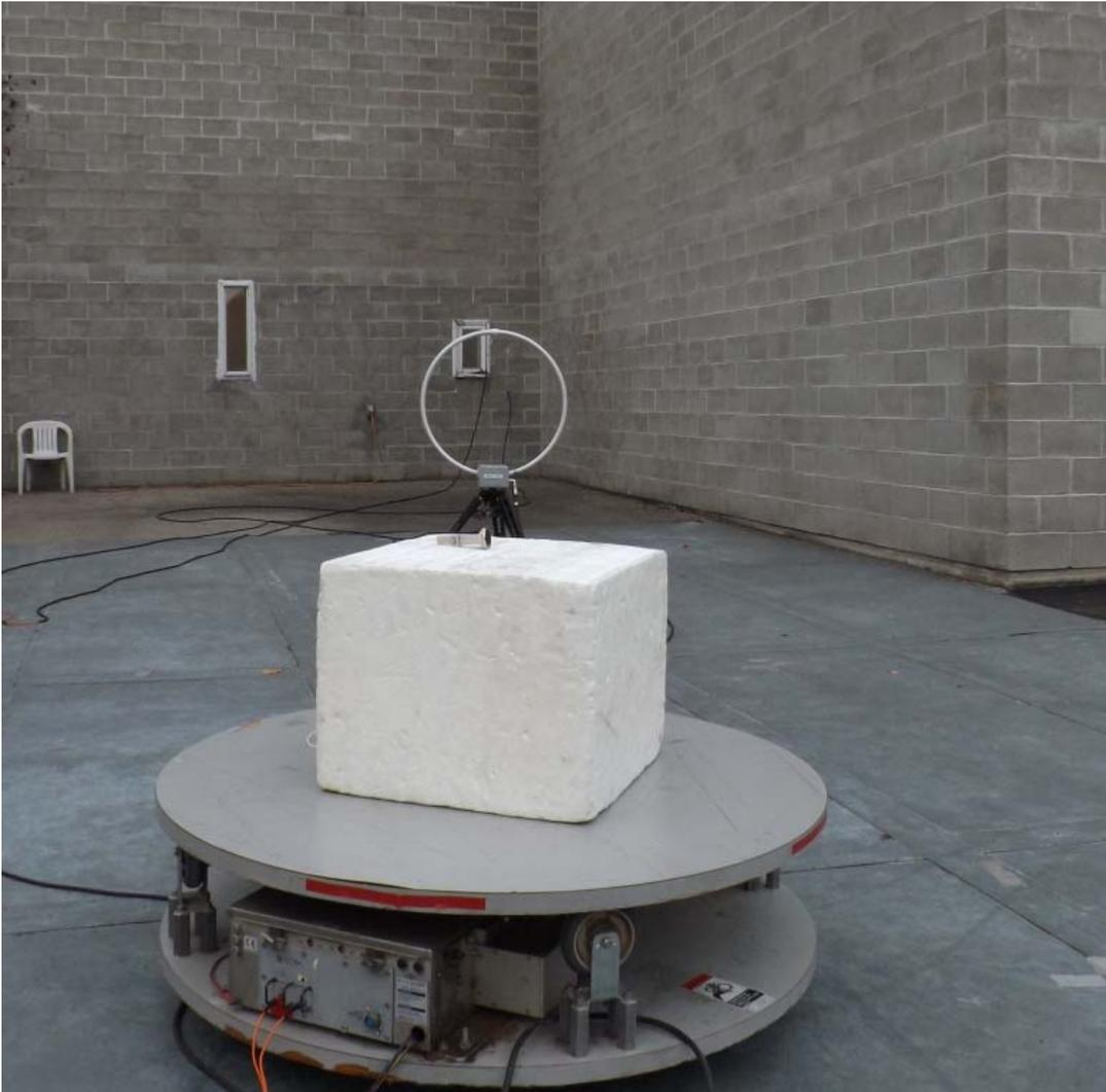
**Figure E20.3 – Setup Photo – Radiated Measurements 30 – 1000MHz**
