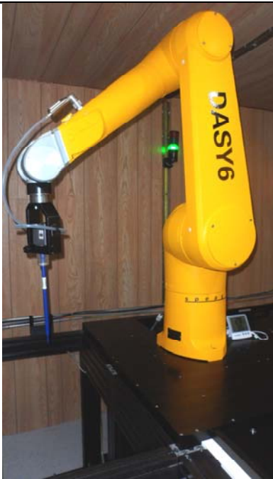
DASY 6 SAR System with SAM Phantom
