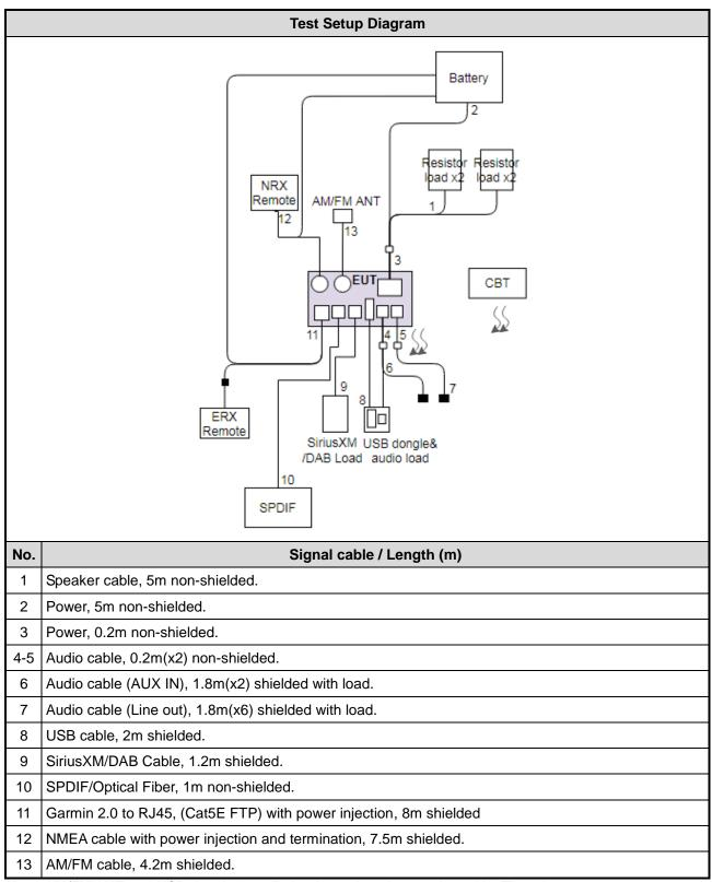
Note: AM/FM ANT and USB dongle & audio load are placed on testing table. The others are on remote testing area.
