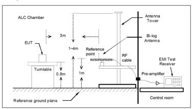
Radiated measurements setup f > 1-18 GHz
