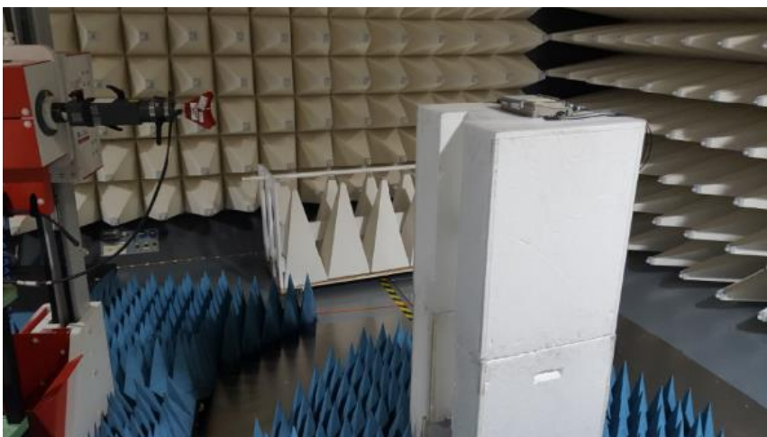
Figure D7. High Range Radiated Emission test setup 3
