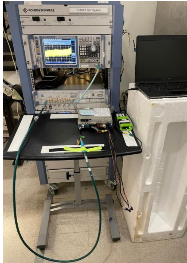
Figure B3. Conducted test setup
