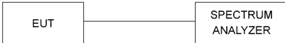
Figure 1 - Bandwidth Measurements Test Setup
