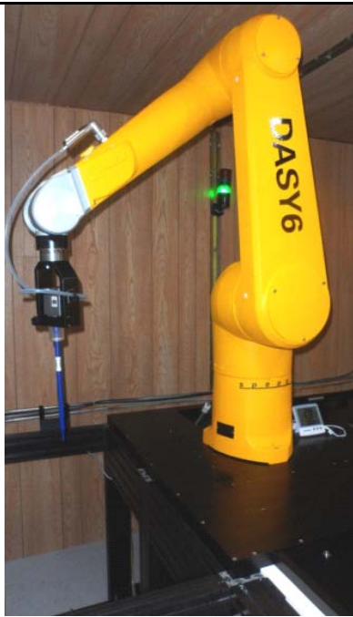
DASY 6 SAR System with SAM Phantom
