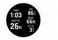
In-dive screen: Displays the information about the current dive, including the elapsed time, current and maximum depth, heart rate data, and rate ascent or descent.
