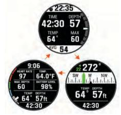
**Dive stopwatch**: Displays the bottom time stopwatch; current, maximum, and average depth; and rate of ascent or decent (*Using the Dive Stopwatch*, page 6).
