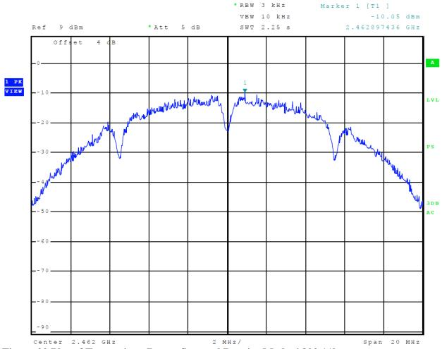
Figure 20 Plot of Transmitter Power Spectral Density Mode 6 802.11b
