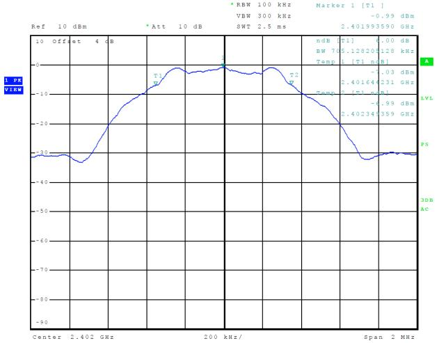
Figure 13 Plot of 6-dB Occupied Bandwidth Mode 2 BLE
