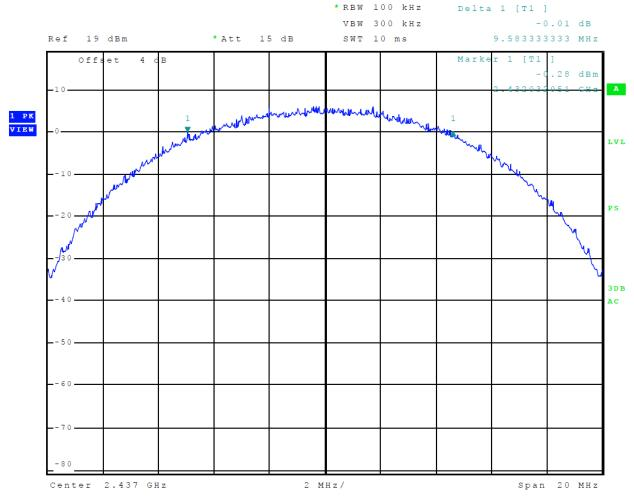
Figure 15 Plot of 6-dB Occupied Bandwidth Mode 3 802.11b
