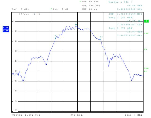
Figure 14 Plot of 99% Occupied Bandwidth Mode 2 BLE
