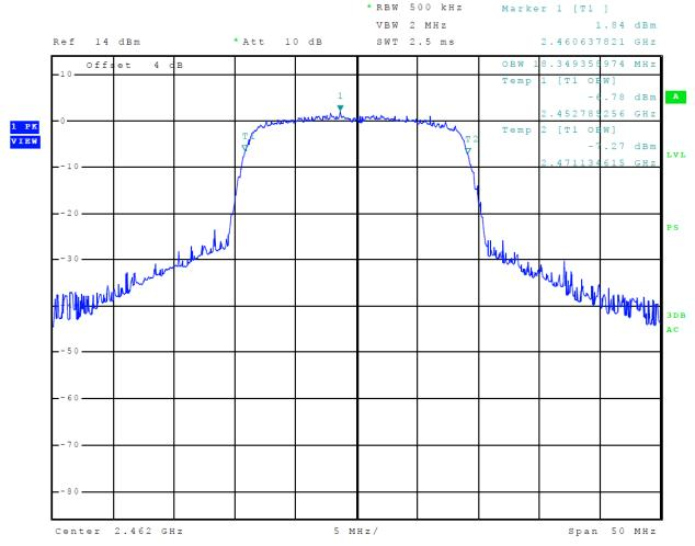
Figure 20 Plot of 99% Occupied Bandwidth Mode 5 802.11n
