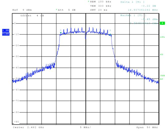
Figure 19 Plot of 6-dB Occupied Bandwidth Mode 5 802.11n
