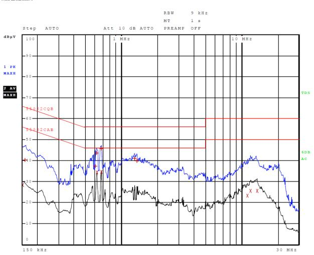
Figure 1 AC Line Conducted emissions of EUT line 1 (Configuration #3, EUT – 362-00096-00)
