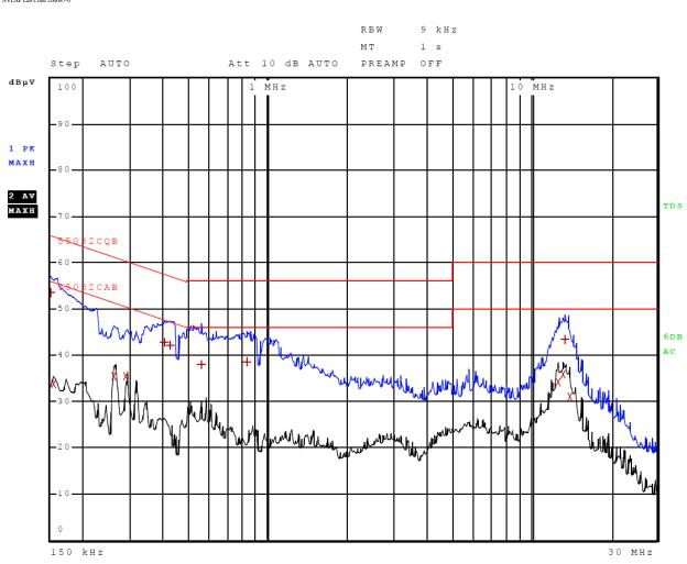
Figure 3 AC Line Conducted emissions of EUT line 1 (Configuration #4, EUT – Computer)
