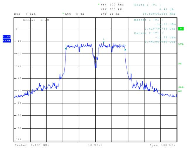
Figure 38 Plot of 6-dB Occupied Bandwidth (Mode 8, 802.11n40)
