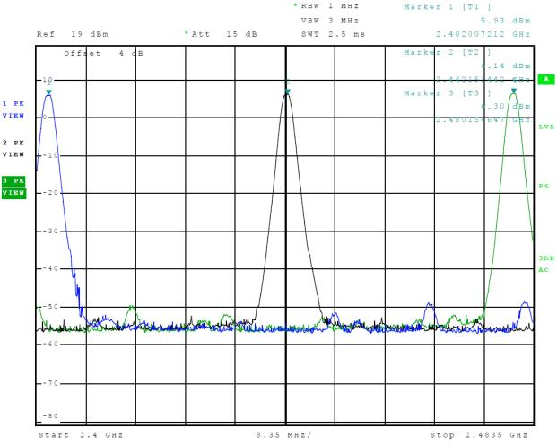
Figure 7 Plot of Transmitter Operation in 2402-2480 MHz (Mode 4, BLE)
