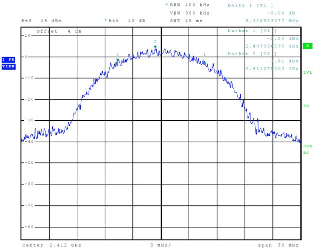
Figure 32 Plot of 6-dB Occupied Bandwidth (Mode 5, 802.11b)
