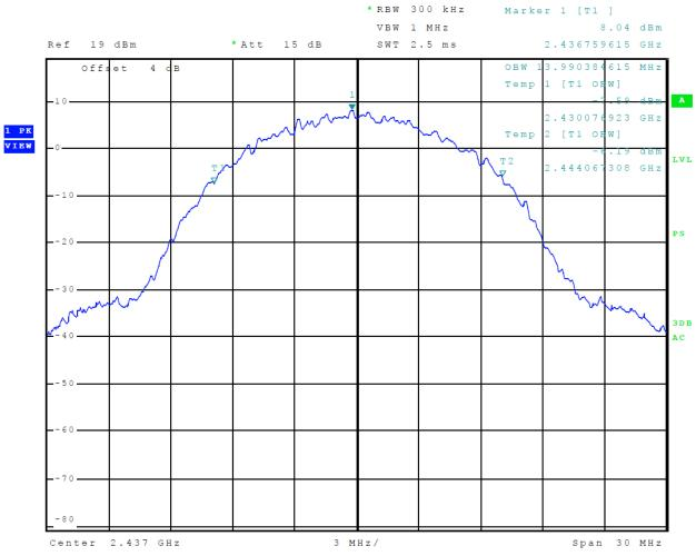
Figure 33 Plot of 99% Occupied Bandwidth (Mode 5, 802.11b)
