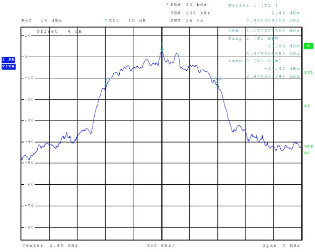
Figure 29 Plot of 99% Occupied Bandwidth (Mode 3, 3EDR)
