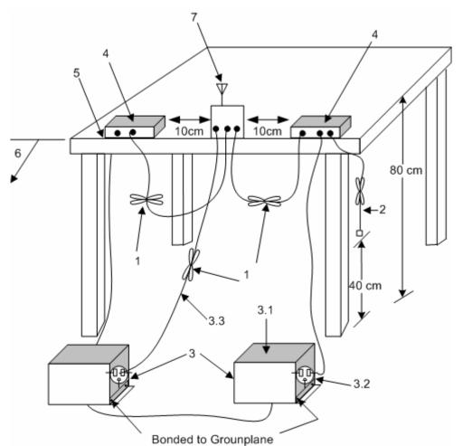
1. Interconnecting cables that hang closer than 40 cm to the ground plane shall be folded back and forth in the center forming a bundle 30 cm to 40 cm long see (see 6.2.3.1).
