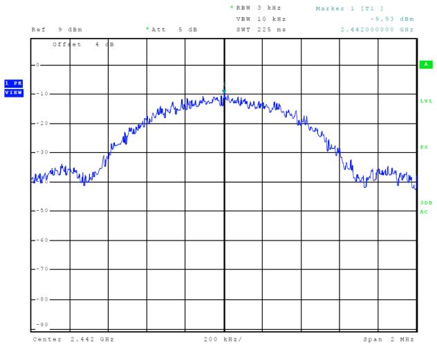
Figure 42 Plot of Transmitter Power Spectral Density (Mode 4, BLE)
