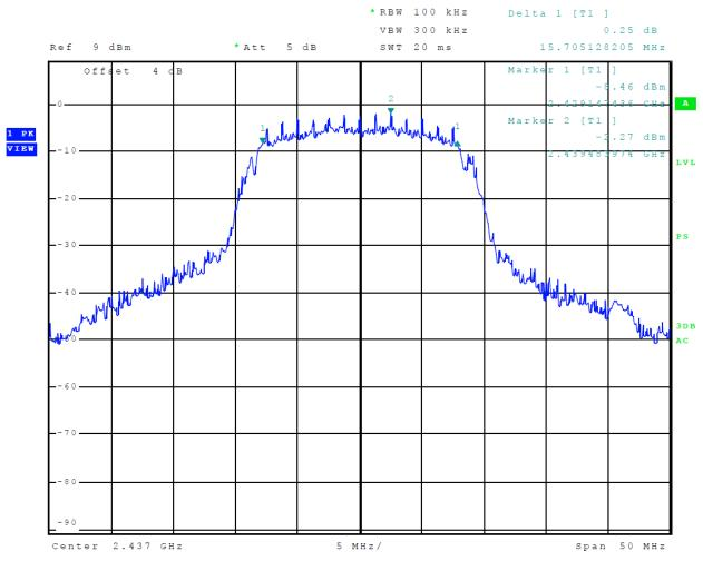
Figure 34 Plot of 6-dB Occupied Bandwidth (Mode 6, 802.11g)
