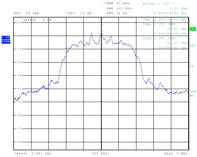
Figure 27 Plot of 99% Occupied Bandwidth (Mode 2, 2EDR)
