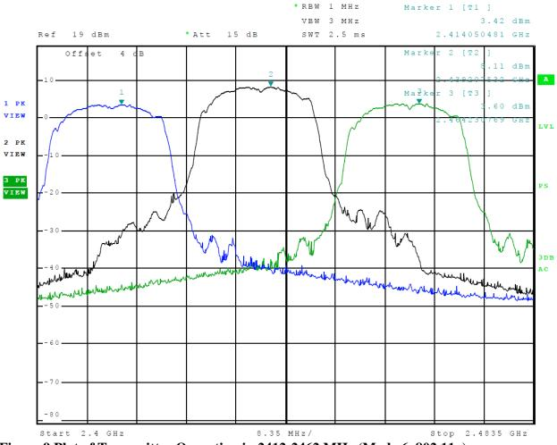
Figure 9 Plot of Transmitter Operation in 2412-2462 MHz (Mode 6, 802.11g)
