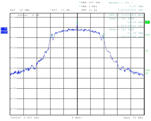
Figure 37 Plot of 99% Occupied Bandwidth (Mode 7, 802.11n)
