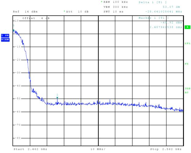
Figure 22 Plot of Transmitter Emissions High Band Edge (Mode 5, 802.11b)
