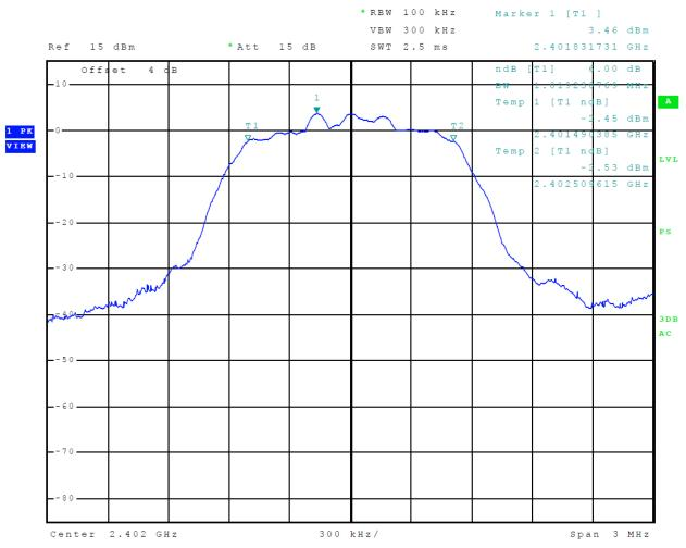
Figure 26 Plot of 6-dB Occupied Bandwidth (Mode 2, 2EDR)
