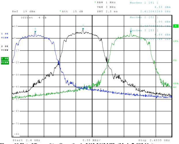
Figure 10 Plot of Transmitter Operation in 2412-2462 MHz (Mode 7, 802.11n)
