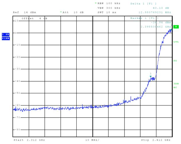
Figure 15 Plot of Transmitter Emissions Low Band Edge (Mode 5, 802.11b)
