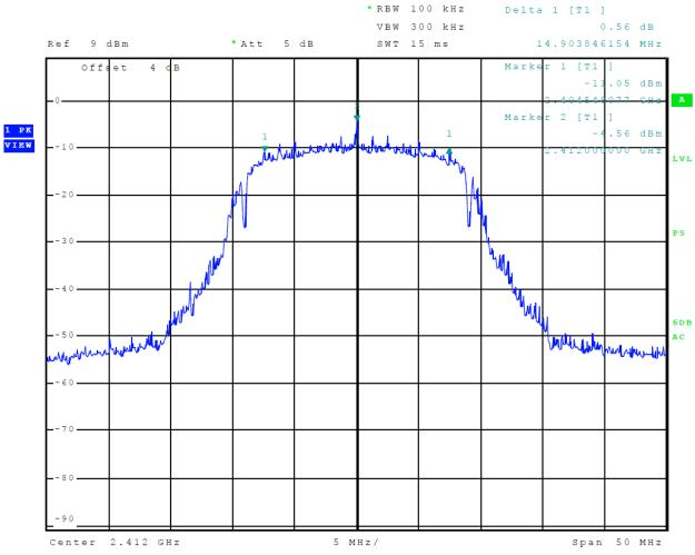
Figure 36 Plot of 6-dB Occupied Bandwidth (Mode 7, 802.11n)
