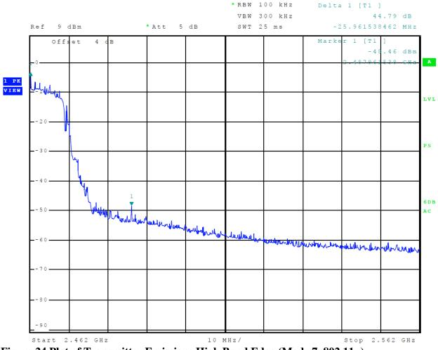
Figure 24 Plot of Transmitter Emissions High Band Edge (Mode 7, 802.11n)
