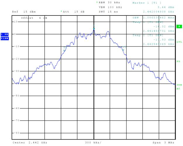
Figure 31 Plot of 99% Occupied Bandwidth (Mode 4, BLE)
