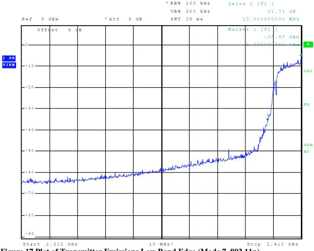
Figure 17 Plot of Transmitter Emissions Low Band Edge (Mode 7, 802.11n)
