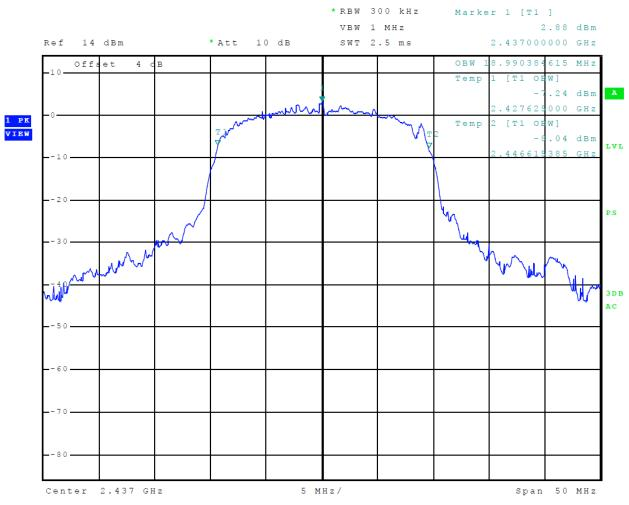
Figure 35 Plot of 99% Occupied Bandwidth (Mode 6, 802.11g)
