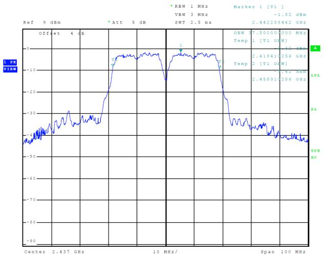
Figure 39 Plot of 99% Occupied Bandwidth (Mode 8, 802.11n40)
