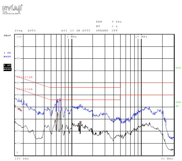
Figure 2 AC Line Conducted emissions of EUT line 2 (Configuration #3, EUT – 362-00096-00)
