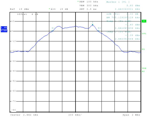
Figure 30 Plot of 6-dB Occupied Bandwidth (Mode 4, BLE)
