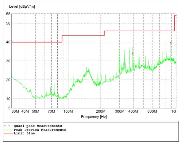
Figure 5 - Radiated Emissions Plot, Low Channel
