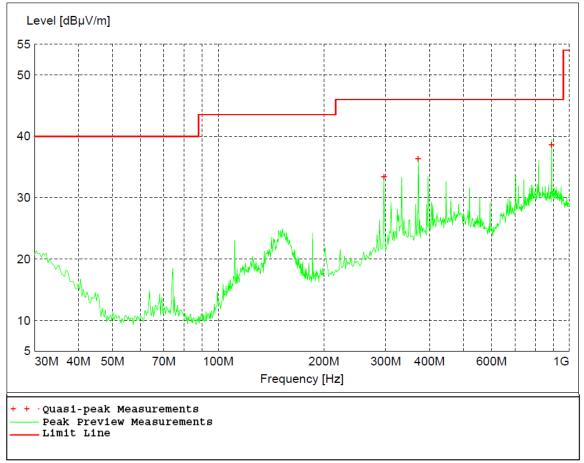
Figure 7 - Radiated Emissions Plot, High Channel
