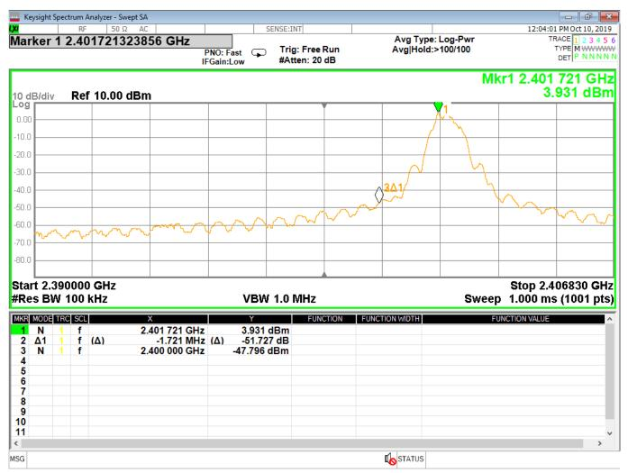
Figure 9 - Band-edge Measurement, Low Channel, Fundamental, Peak
