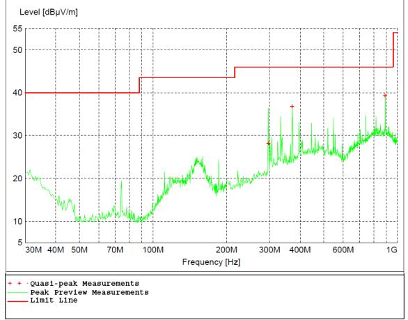
Figure 6 - Radiated Emissions Plot, Mid Channel
