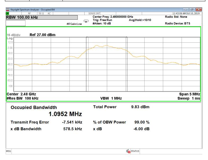
Figure 19 - High Channel, GFSK
