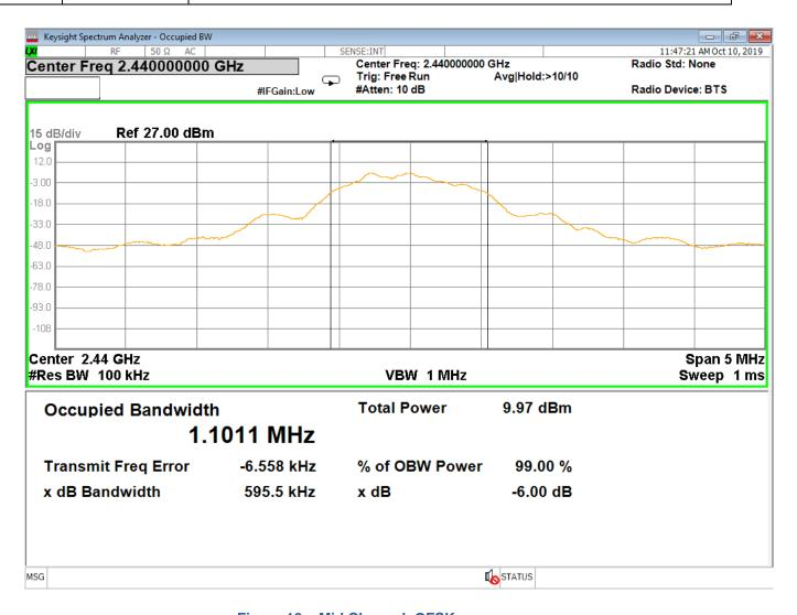
Figure 18 – Mid Channel, GFSK
