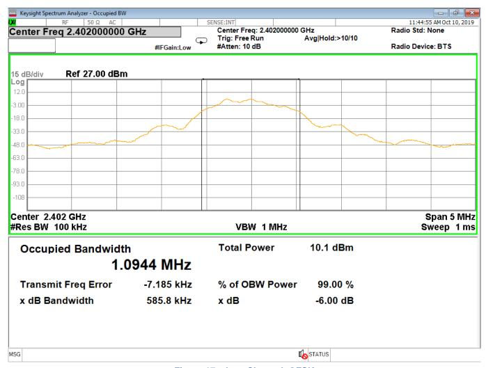
Figure 17 - Low Channel, GFSK
