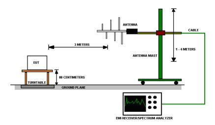
Figure 3 - Radiated Emissions Test Setup
