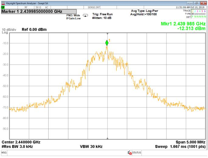
Figure 13 - Power Spectral Density, Mid Channel, GFSK
