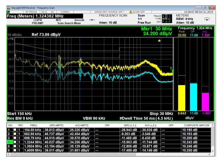
Figure 15 - Conducted Emissions, Line
