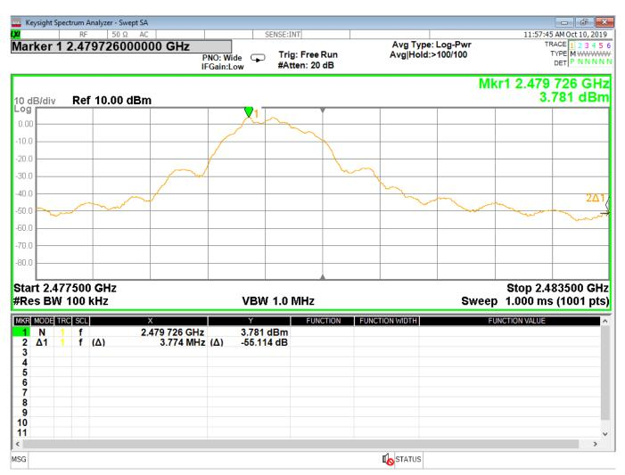
Figure 11 - Band-edge Measurement, High Channel, Fundamental, Peak
