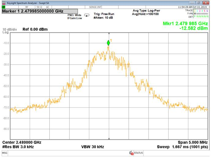
Figure 14 - Power Spectral Density, High Channel, GFSK
