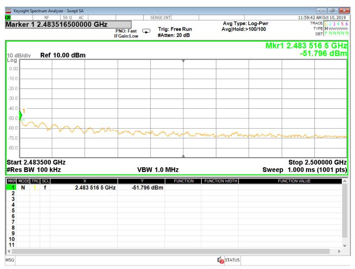
Figure 10 - Band-edge Measurement, High Channel, Restricted Frequency, Peak
