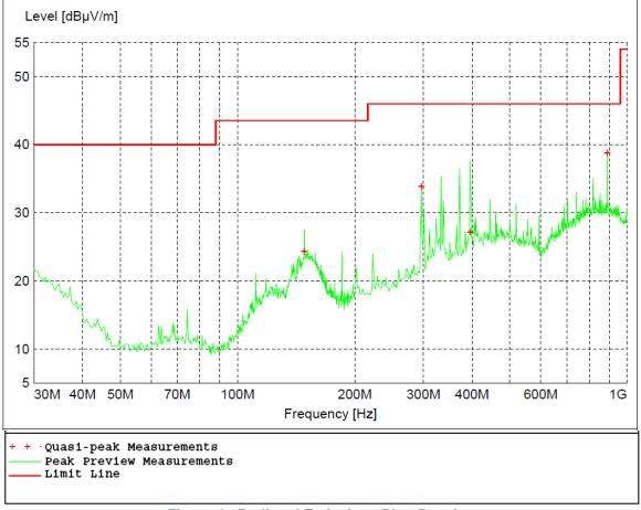
Figure 4 - Radiated Emissions Plot, Receive
