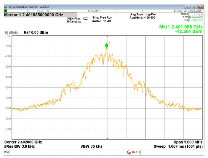
Figure 12 - Power Spectral Density, Low Channel, GFSK
