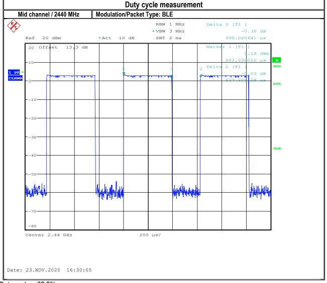
Duty cycle = 62.2%Duty cycle correction factor =  $10*\log(1/0.622) = 2.06$  dB
