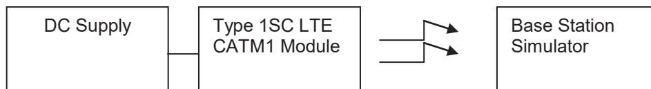
Setup for radiated measurements
