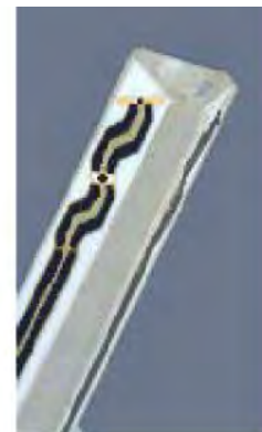
Figure 2.3 Probe Thick-Film Technique
