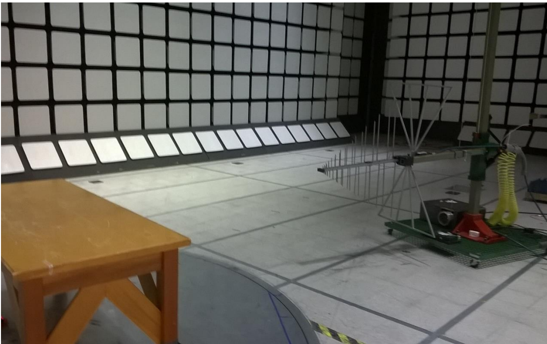
Figure 2 - Radiated Emissions Test Setup, 30 MHz - 1 GHz (EUT not shown. Photo intended to show equipment setup)
