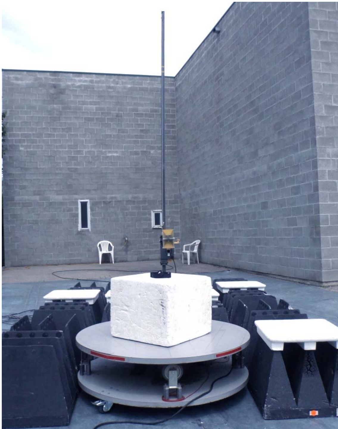
Figure E20.4 – Setup Photo – Radiated Measurements > 1GHz – Horizontal
