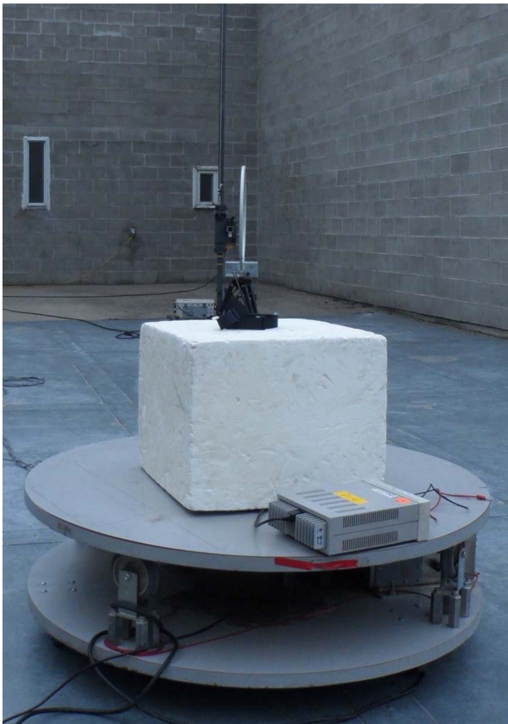
Figure E20.7 – Setup Photo – Radiated Measurements < 30MHz – Side
