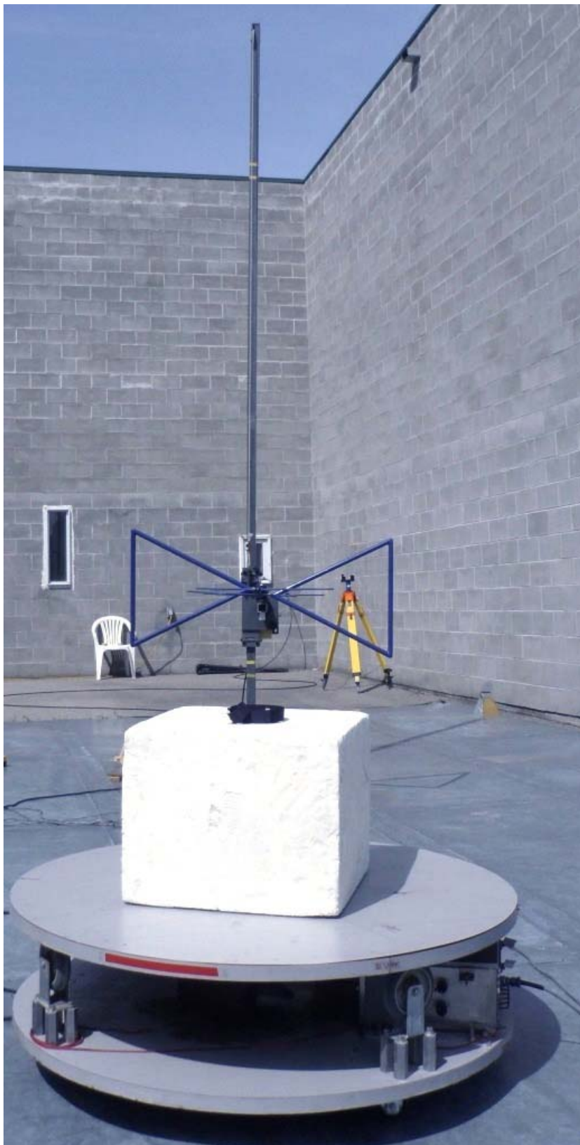
Figure E20.2 – Setup Photo – Radiated Measurements – 30 to 1000MHz
