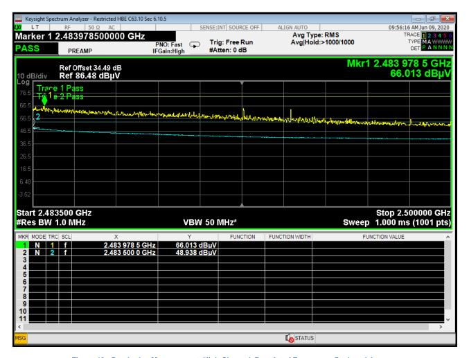
Figure 46 - Band-edge Measurement, High Channel, Restricted Frequency, Peak and Average
