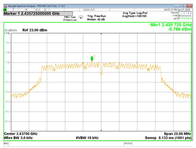
Figure 57 - Power Spectral Density, Mid Channel, 802.11g
