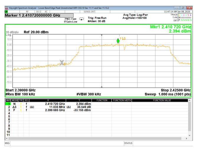
Figure 47 - Band-edge Measurement, Low Channel, Fundamental, Peak
