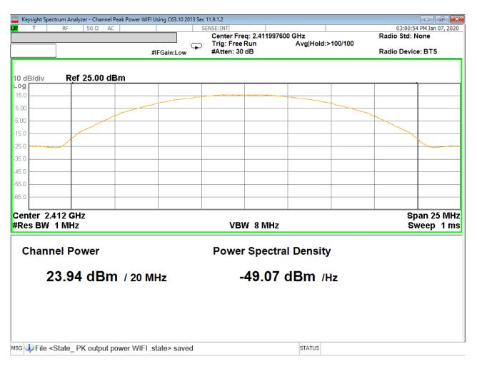
Figure 7 – Peak Output Power, Low Channel, 802.11b
