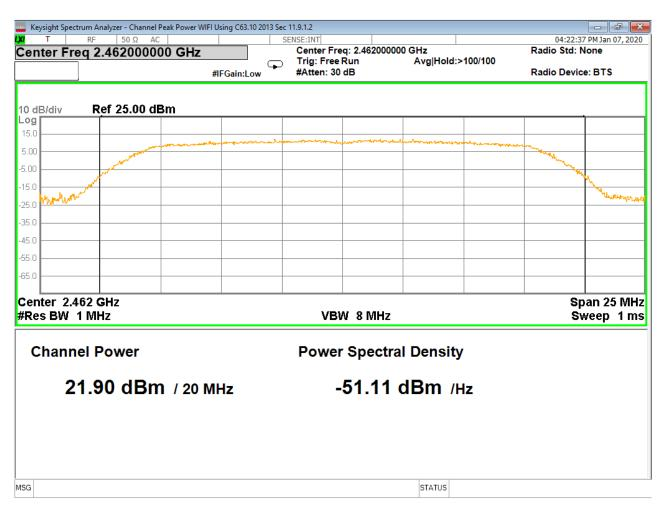
Figure 12 - Peak Output Power, High Channel, 802.11g
