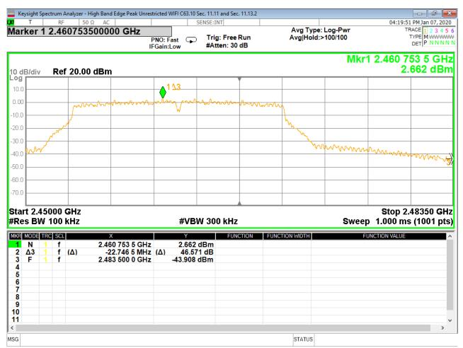
Figure 43 - Band-edge Measurement, High Channel, Fundamental, Peak
