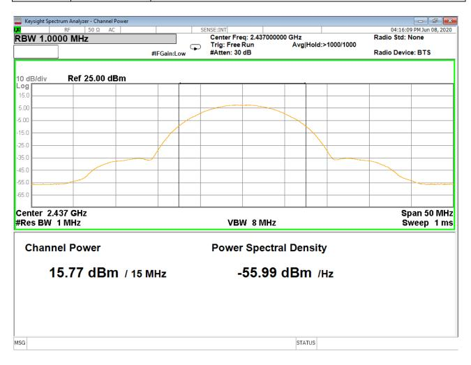
Figure 17 – Average Output Power, Mid Channel, 802.11b
