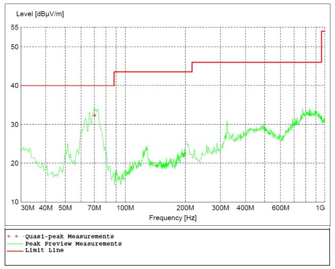
Figure 4 - Radiated Emissions Plot, 802.11g
