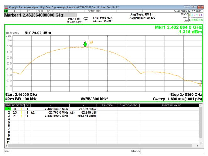
Figure 38 - Band-edge Measurement, High Channel, Fundamental, Average
