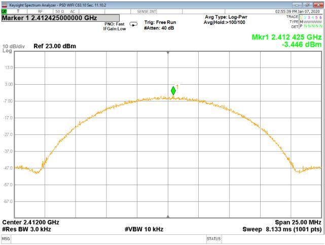
Figure 53 - Power Spectral Density, Low Channel, 802.11b
