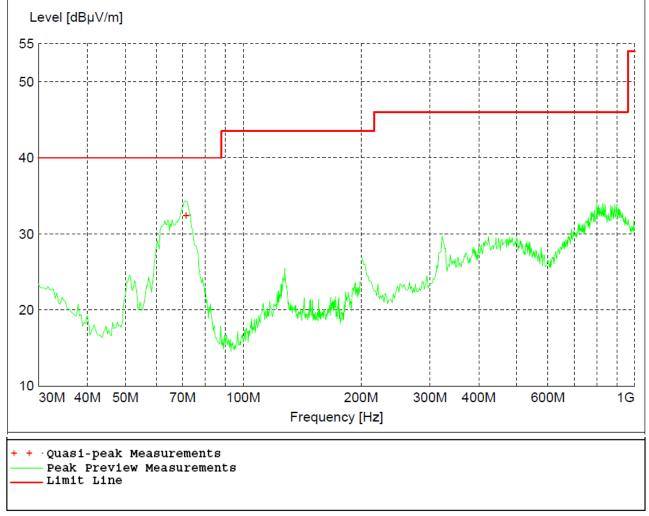
Figure 5 - Radiated Emissions Plot, 802.11n
