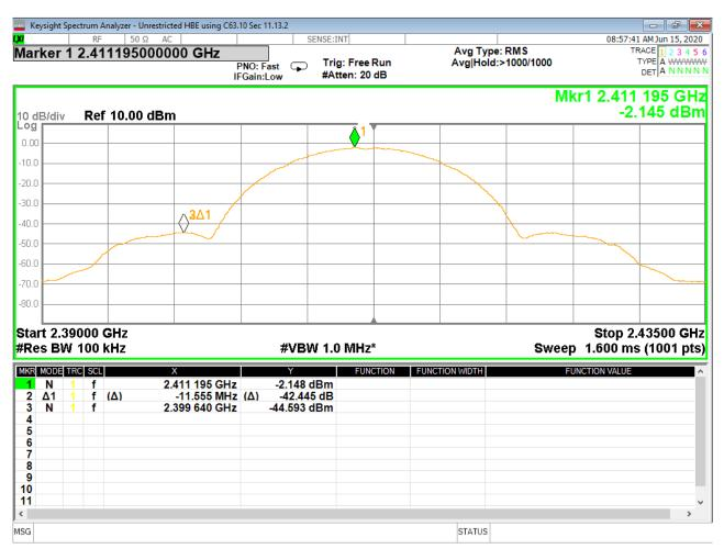
Figure 36 - Band-edge Measurement, Low Channel, Fundamental, Average
