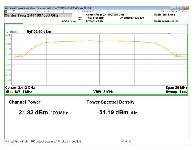
Figure 10 - Peak Output Power, Low Channel, 802.11g
