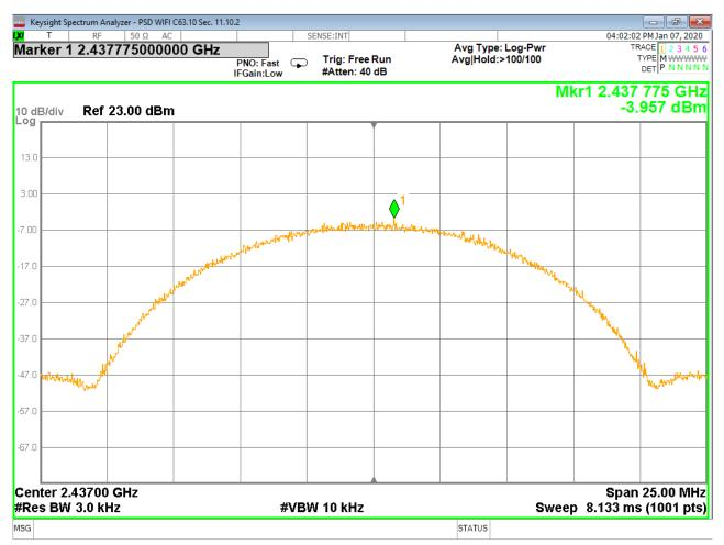
Figure 54 - Power Spectral Density, Mid Channel, 802.11b
