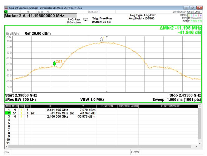
Figure 35 - Band-edge Measurement, Low Channel, Fundamental, Peak
