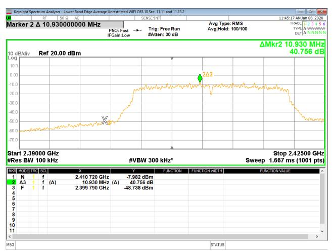
Figure 48 - Band-edge Measurement, Low Channel, Fundamental, Average
