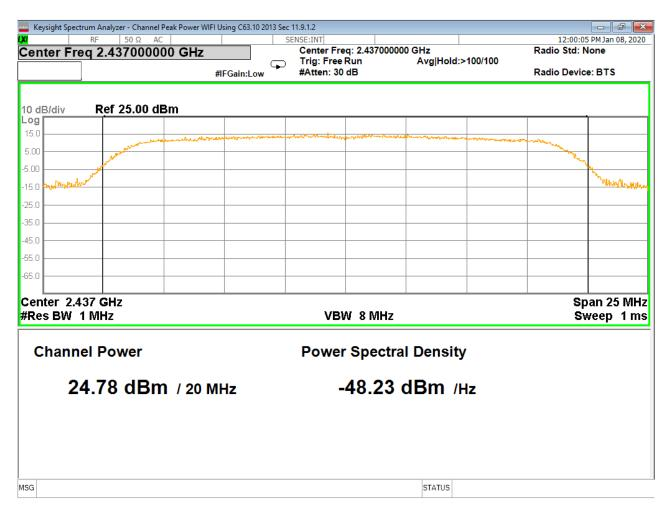
Figure 14 - Peak Output Power, Mid Channel, 802.11n
