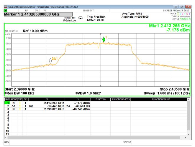
Figure 42 - Band-edge Measurement, Low Channel, Fundamental, Average
