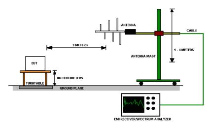
Figure 1 - Radiated Emissions Test Setup
