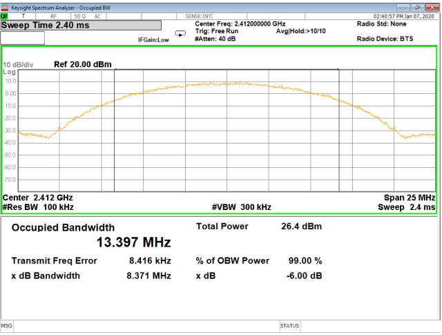
Figure 26 - Bandwidth, Low Channel, 802.11b
