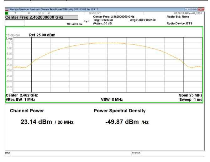
Figure 9 - Peak Output Power, High Channel, 802.11b
