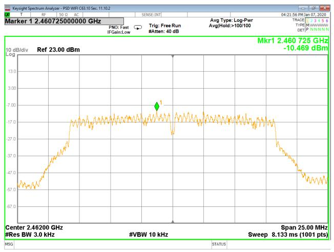
Figure 58 - Power Spectral Density, High Channel, 802.11g
