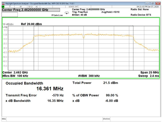
Figure 31 - Bandwidth, High Channel, 802.11g
