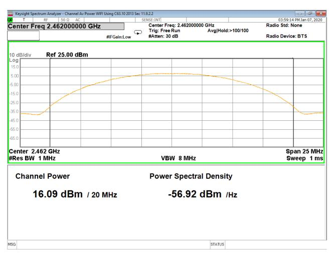
Figure 18 - Average Output Power, High Channel, 802.11b
