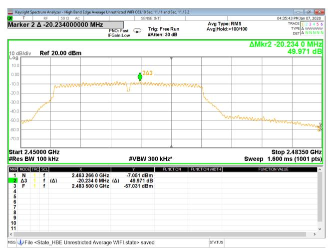
Figure 44 - Band-edge Measurement, High Channel, Fundamental, Average
