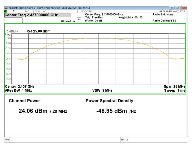
Figure 8 - Peak Output Power, Mid Channel, 802.11b
