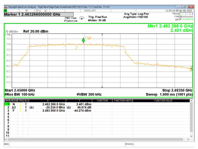
Figure 49 - Band-edge Measurement, High Channel, Fundamental, Peak
