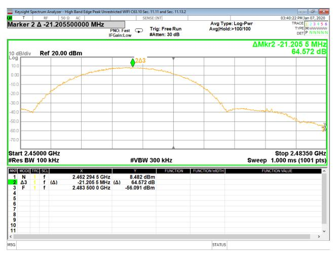
Figure 37 - Band-edge Measurement, High Channel, Fundamental, Peak
