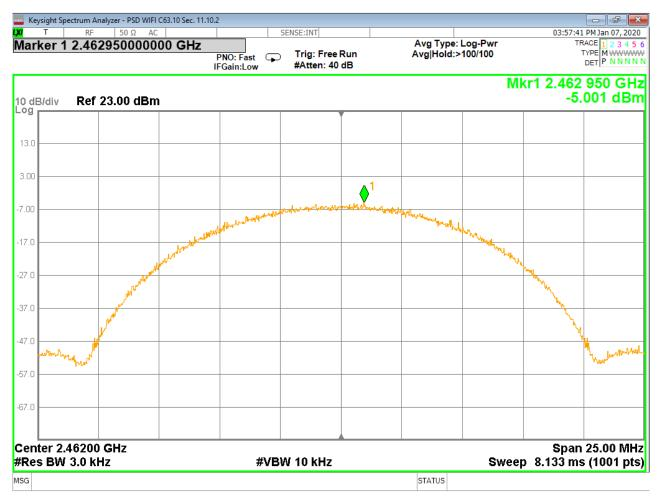
Figure 55 - Power Spectral Density, High Channel, 802.11b
