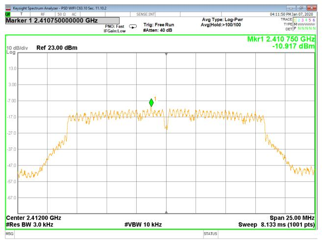
Figure 56 - Power Spectral Density, Low Channel, 802.11g
