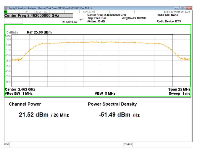
Figure 15 - Peak Output Power, High Channel, 802.11n
