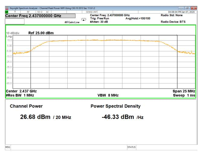
Figure 11 - Peak Output Power, Mid Channel, 802.11g
