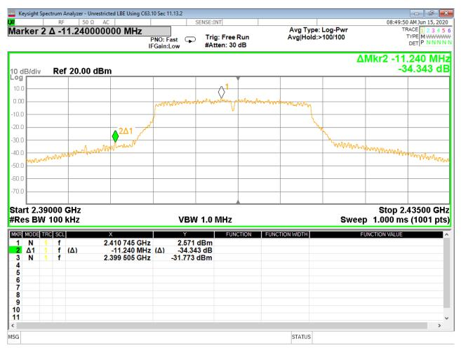
Figure 41 - Band-edge Measurement, Low Channel, Fundamental, Peak
