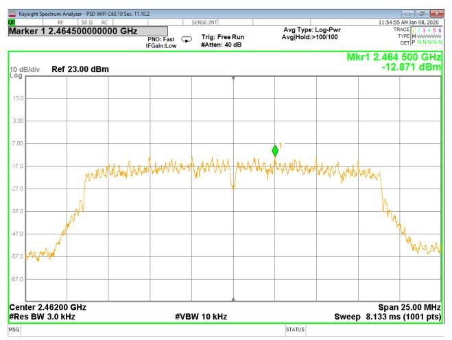
Figure 61 - Power Spectral Density, High Channel, 802.11n
