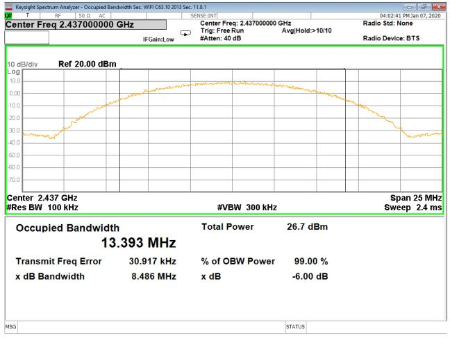
Figure 27 - Bandwidth, Mid Channel, 802.11b
