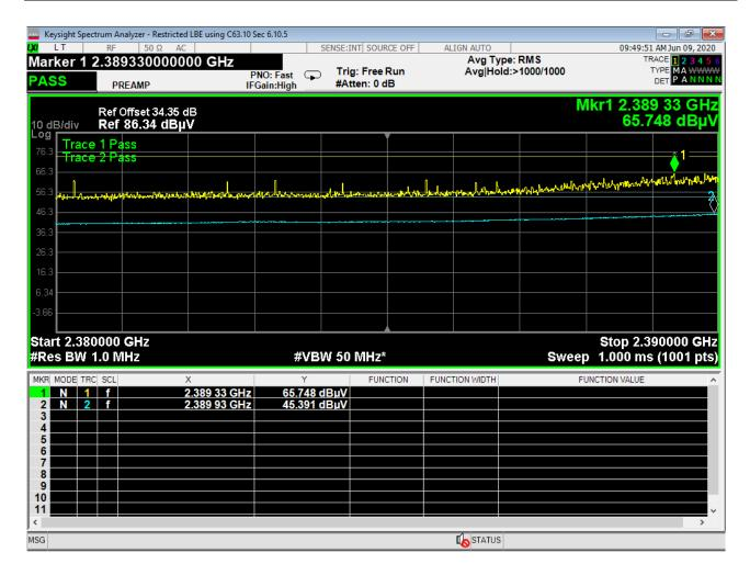
Figure 51 - Band-edge Measurement, Low Channel, Restricted Frequency, Peak and Average
