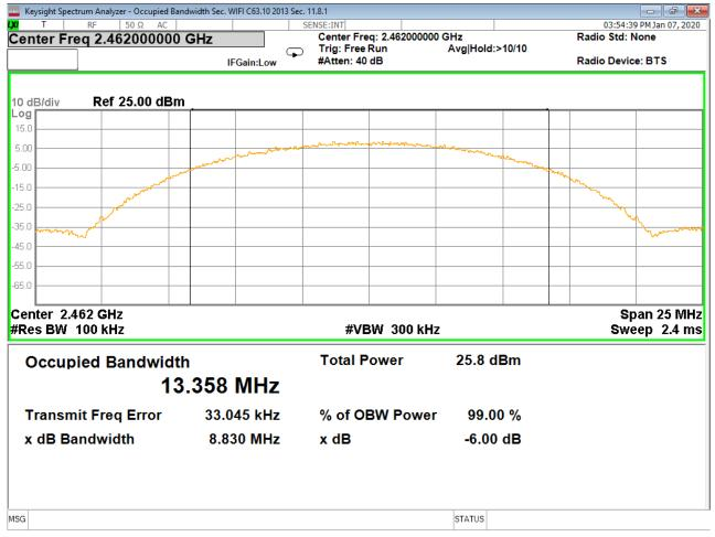
Figure 28 - Bandwidth, High Channel, 802.11b
