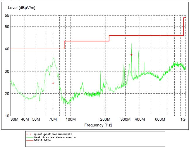
Figure 2 - Radiated Emissions Plot, Receive
