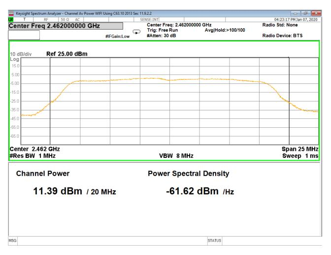
Figure 21 - Average Output Power, High Channel, 802.11g
