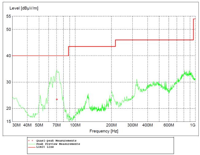
Figure 3 - Radiated Emissions Plot, 802.11b
