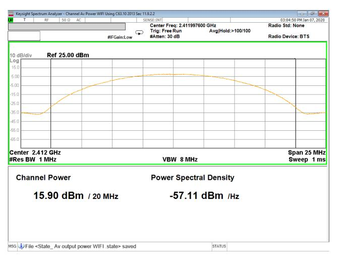
Figure 16 – Average Output Power, Low Channel, 802.11b
