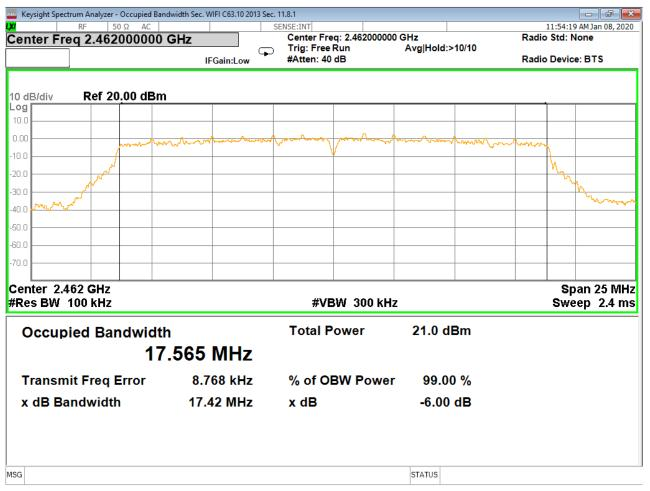
Figure 34 - Bandwidth, High Channel, 802.11n
