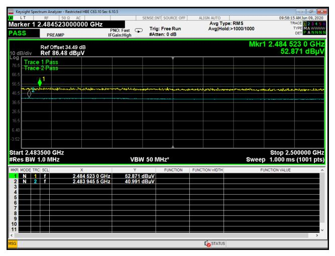
Figure 40 - Band-edge Measurement, High Channel, Restricted Frequency, Peak and Average
