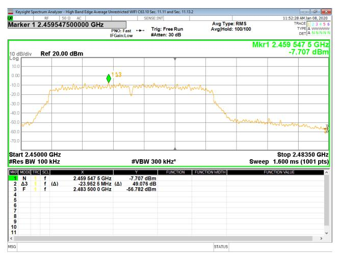
Figure 50 - Band-edge Measurement, High Channel, Fundamental, Average
