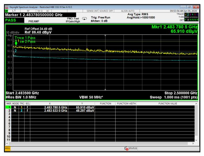
Figure 52 - Band-edge Measurement, High Channel, Restricted Frequency, Peak and Average
