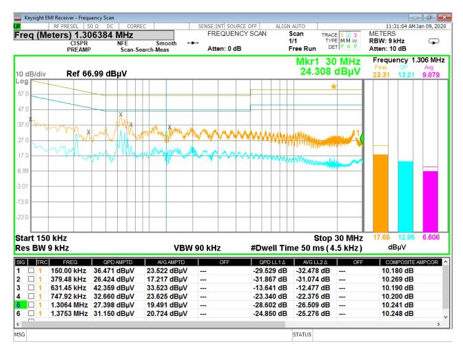
Figure 62 - Conducted Emissions Plot, Line
