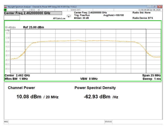
Figure 24 - Average Output Power, High Channel, 802.11n
