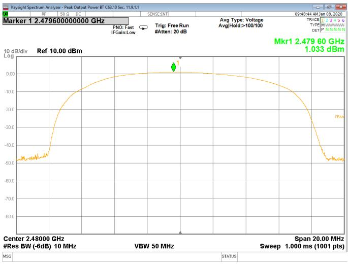
Figure 4 - Output Power, High Channel, BT EDR 2MB
