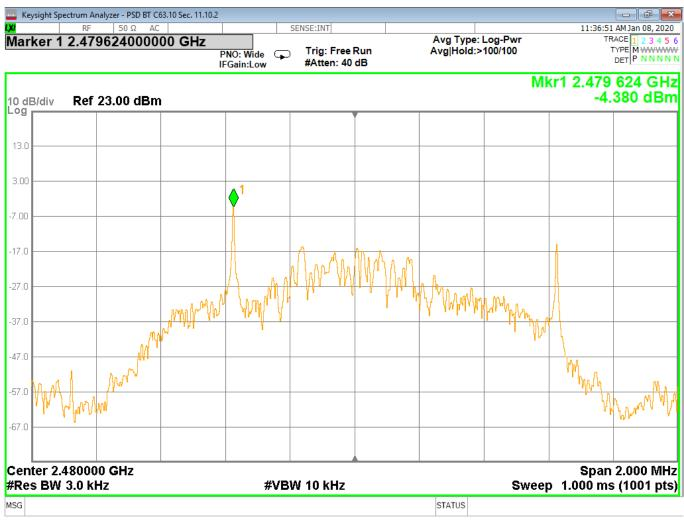
Figure 44 - Power Spectral Density, High Channel, BT EDR 3MB
