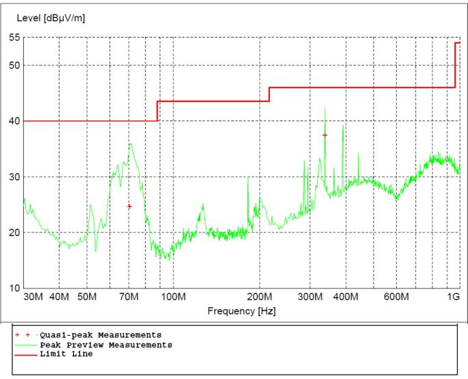
Figure 25 - Radiated Emissions Plot, Receive
