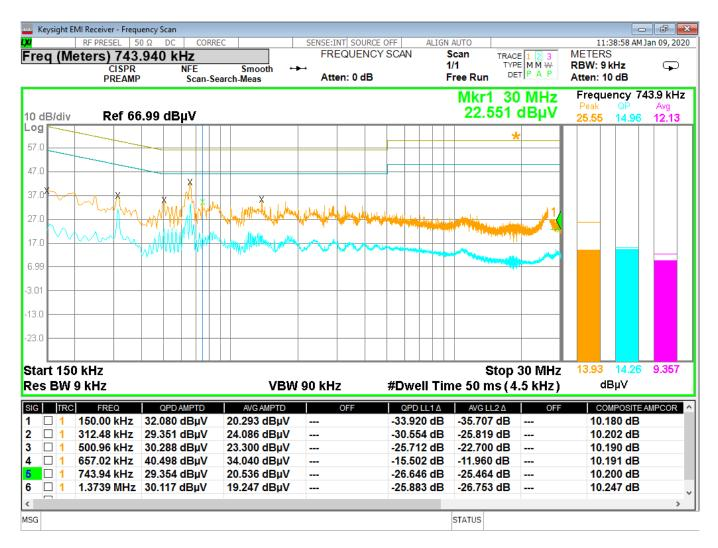
Figure 45 - Conducted Emissions, Line
