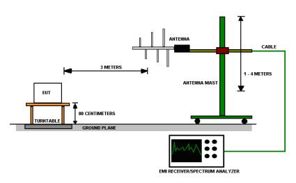
Figure 24 - Radiated Emissions Test Setup
