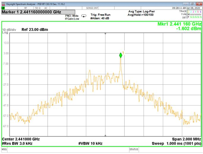
Figure 37 - Power Spectral Density, Mid Channel, BT BR (GFSK)
