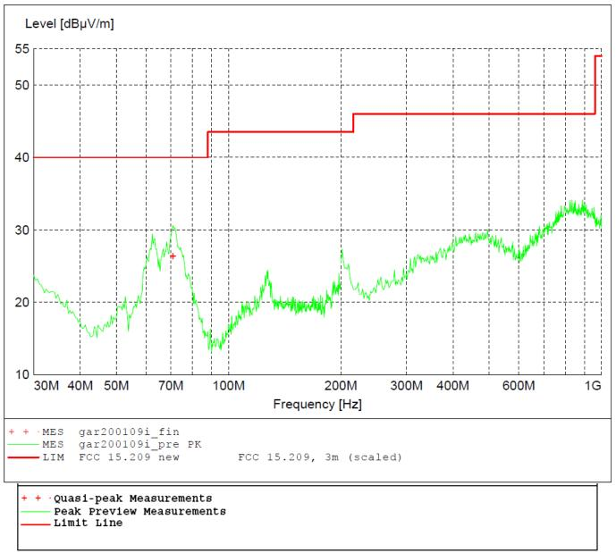
Figure 27 - Radiated Emissions Plot, 3EDR
