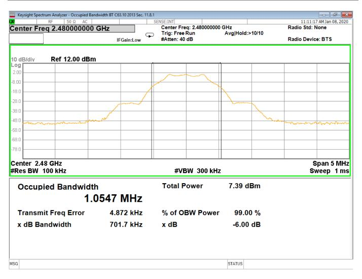
Figure 4 - Occupied Bandwidth, High Channel, GMSK
