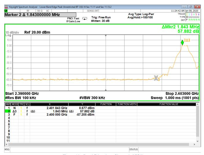
Figure 16 - Band Edge, Low Channel, GFSK
