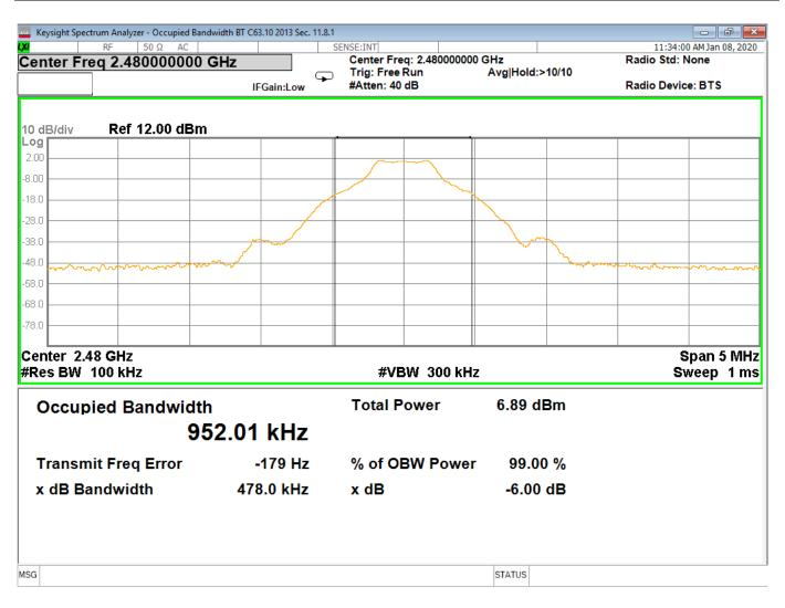
Figure 7 - Occupied Bandwidth, High Channel, GFSK
