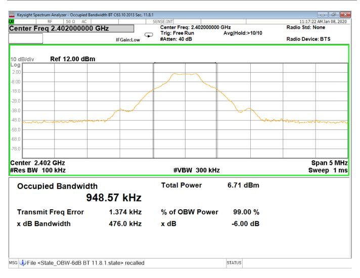
Figure 5 - Occupied Bandwidth, Low Channel, GFSK
