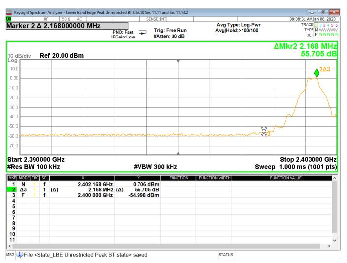
Figure 20 -Band Edge, Low Channel, BTBR
