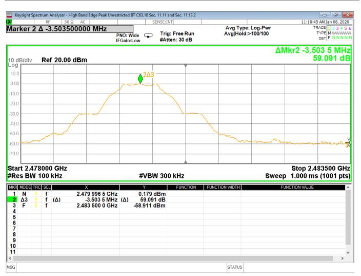
Figure 19 - Band Edge Measurement, High Channel, GMSK
