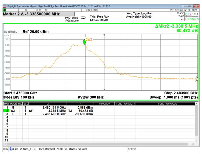
Figure 21 - Band Edge Measurement, High Channel, BTBR
