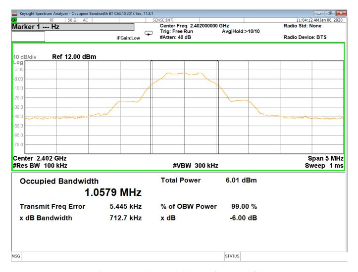
Figure 2 - Occupied Bandwidth, Low Channel, GMSK
