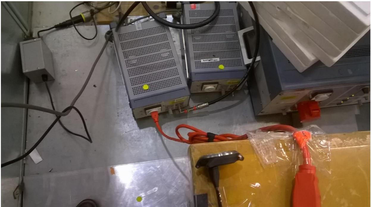
Figure 4 - Conducted Emissions Test Setup (AC power supply is on table.)
