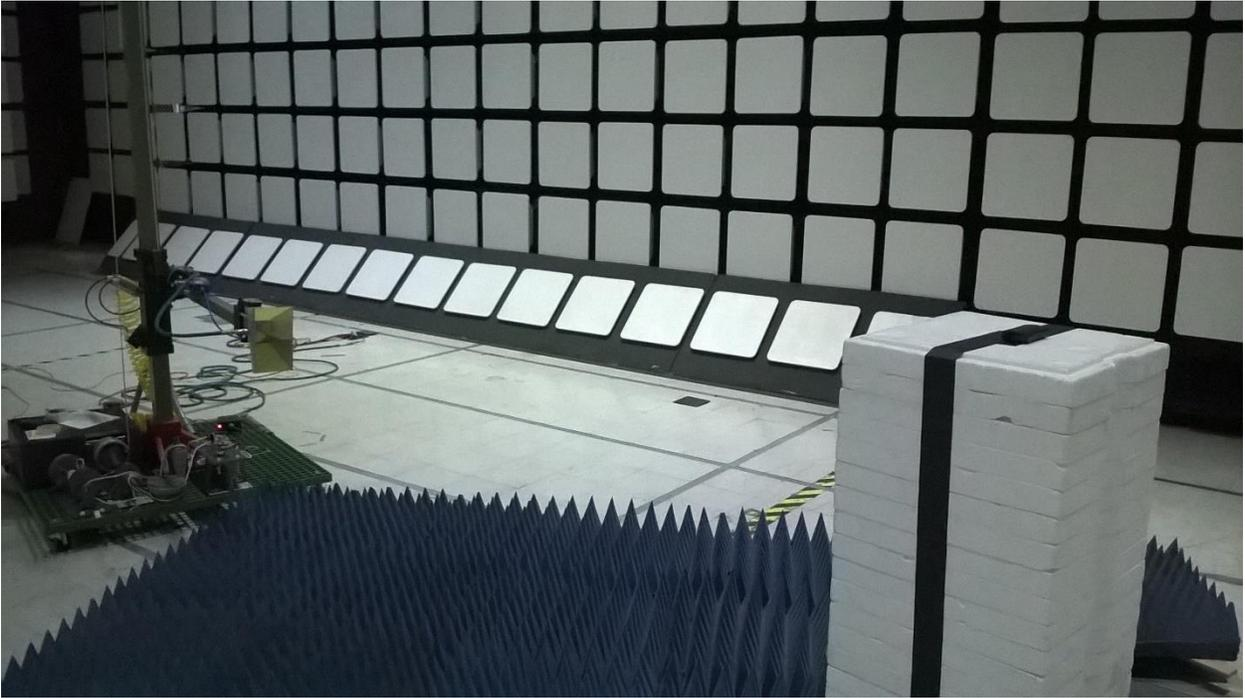
*Figure 1 - Radiated Emissions Test Setup, 1 - 25 GHz*
