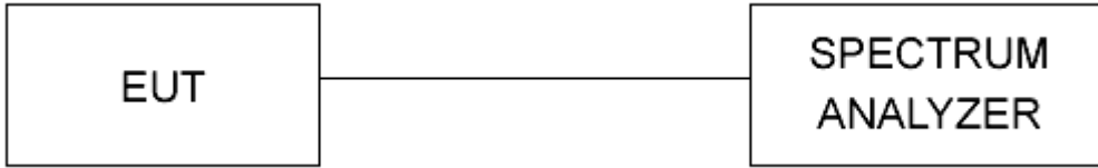
Figure 9 - Bandwidth Measurements Test Setup
