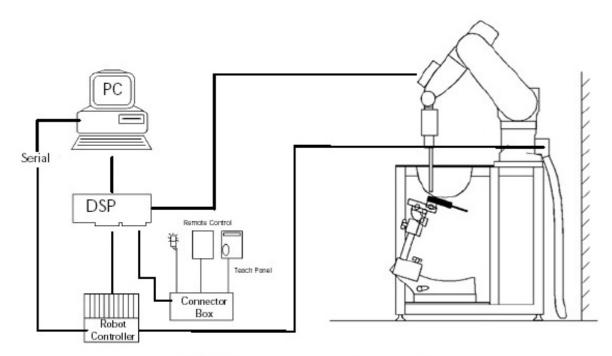
Figure 2.1 SAR Measurement System Setup
