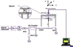
Figure 7.1 Dipole Verification Test Setup
