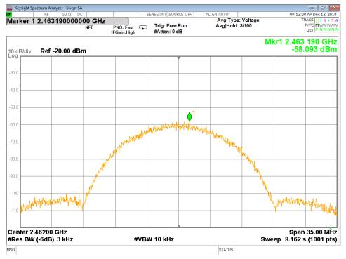
Figure 51 - Power Spectral Density, High Channel, 802.11b
