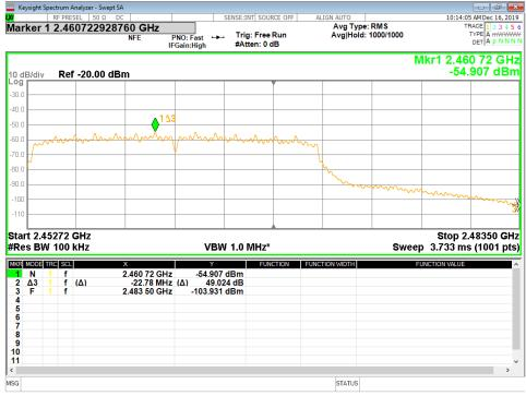
Figure 47 - Band-edge Measurement, High Channel, Fundamental, Average
