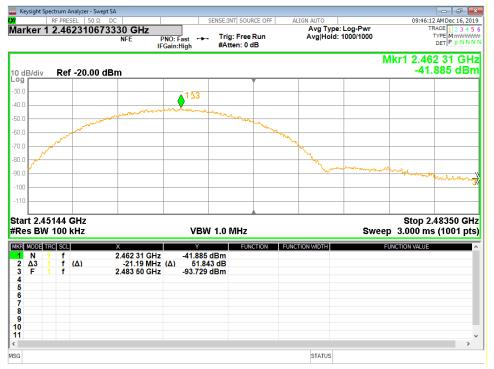
Figure 29 - Band-edge Measurement, High Channel, Fundamental, Peak
