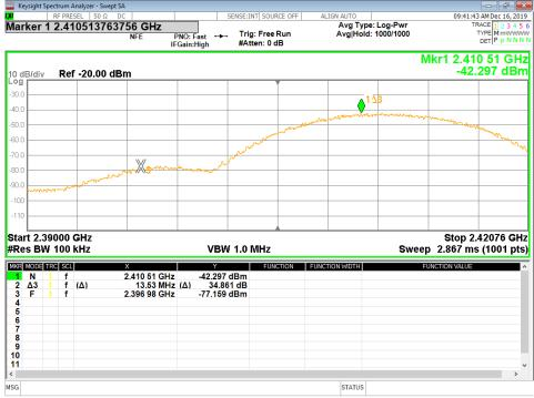
Figure 25 - Band-edge Measurement, Low Channel, Fundamental, Peak
