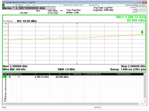
Figure 40 - Band-edge Measurement, Low Channel, Restricted Frequency, Peak
