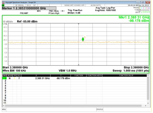
Figure 24 - Band-edge Measurement, Low Channel, Restricted Frequency, Peak
