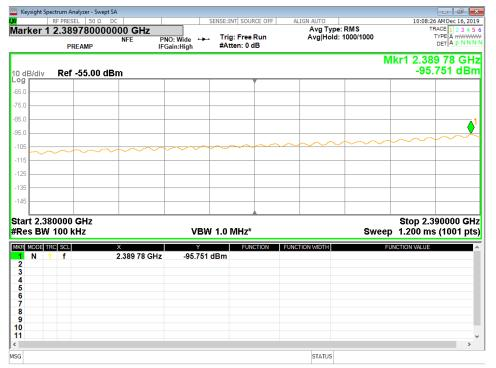
Figure 34 - Band-edge Measurement, Low Channel, Restricted Frequency, Average
