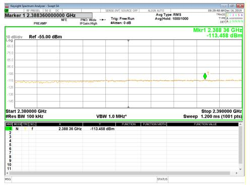
Figure 26 - Band-edge Measurement, Low Channel, Restricted Frequency, Average
