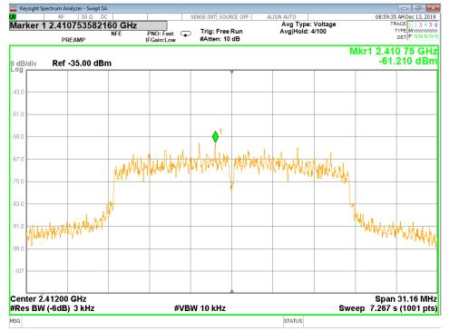
Figure 55 - Power Spectral Density, Low Channel, 802.11n
