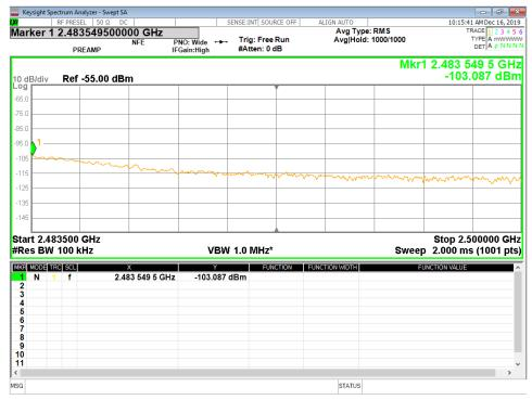
Figure 46 - Band-edge Measurement, High Channel, Restricted Frequency, Average
