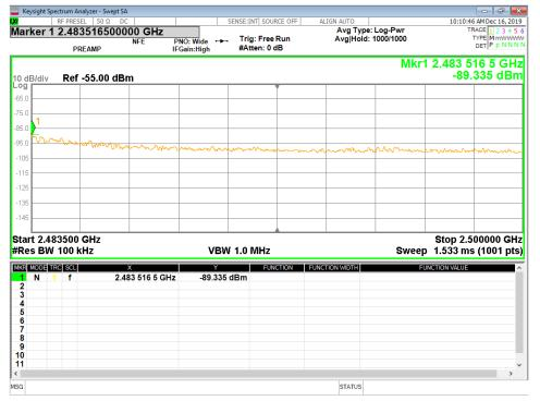
Figure 36 - Band-edge Measurement, High Channel, Restricted Frequency, Peak
