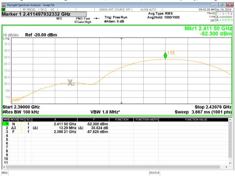
Figure 27 - Band-edge Measurement, Low Channel, Fundamental, Average
