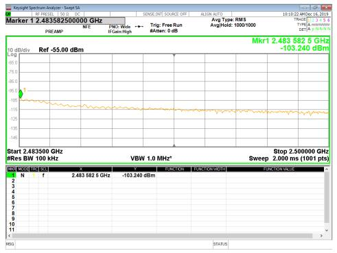
Figure 38 - Band-edge Measurement, High Channel, Restricted Frequency, Average
