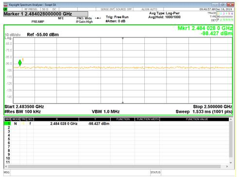
Figure 28 - Band-edge Measurement, High Channel, Restricted Frequency, Peak
