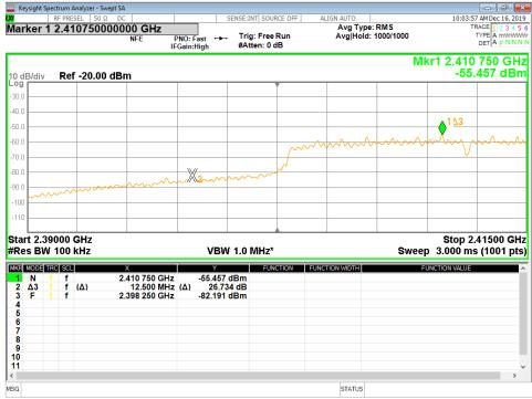
Figure 43 - Band-edge Measurement, Low Channel, Fundamental, Average
