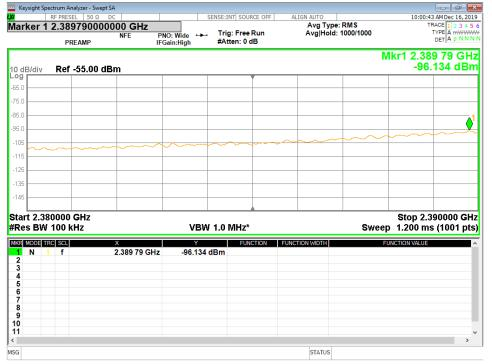
Figure 42 - Band-edge Measurement, Low Channel, Restricted Frequency, Average
