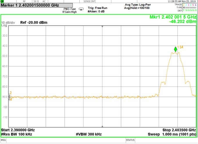
Figure 17 - Band-edge Measurement, Low Channel, Fundamental, Peak, GMSK
