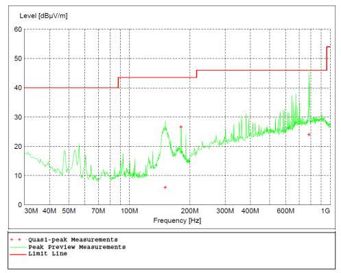
Figure 4 - Radiated Emissions Plot, 802.11g
