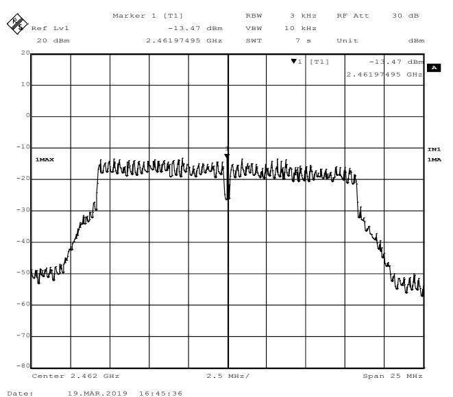
Figure 61 - Power Spectral Density, High Channel, 802.11g
