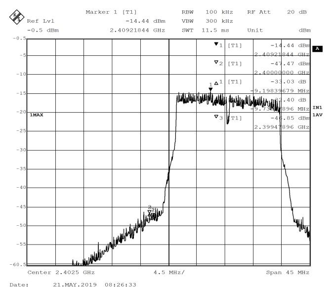
Figure 43 - Band-edge Measurement, Low Channel, Fundamental, Average
