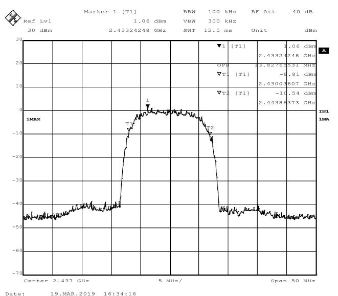
Figure 15 - 99% Occupied Bandwidth, Mid Channel, 802.11b
