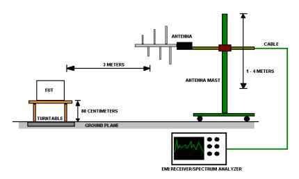
Figure 1 - Radiated Emissions Test Setup
