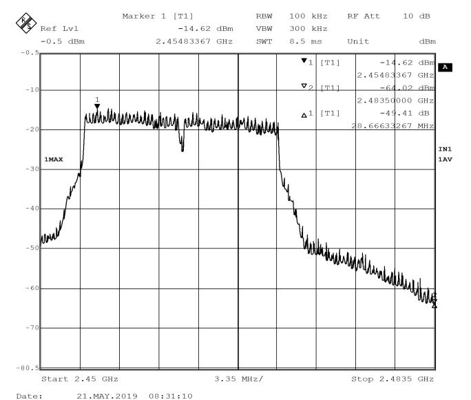
Figure 47 - Band-edge Measurement, High Channel, Fundamental, Average
