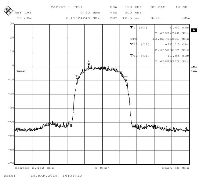
Figure 16 - 99% Occupied Bandwidth, High Channel, 802.11b
