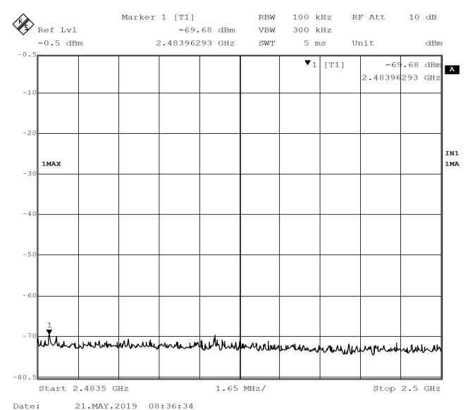
Figure 36 - Band-edge Measurement, High Channel, Restricted Frequency, Peak
