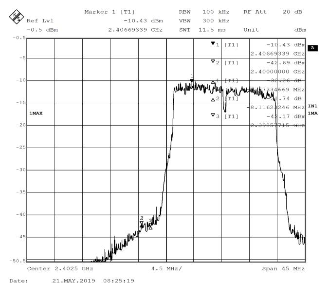
Figure 41 - Band-edge Measurement, Low Channel, Fundamental, Peak
