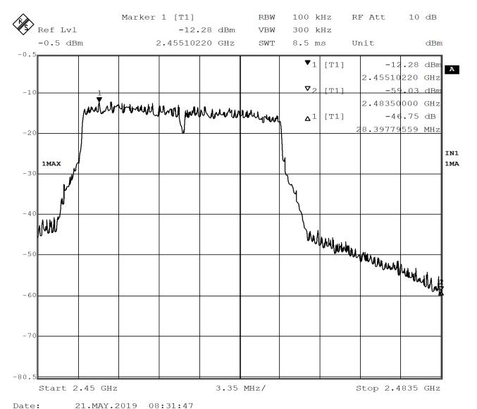
Figure 45 - Band-edge Measurement, High Channel, Fundamental, Peak
