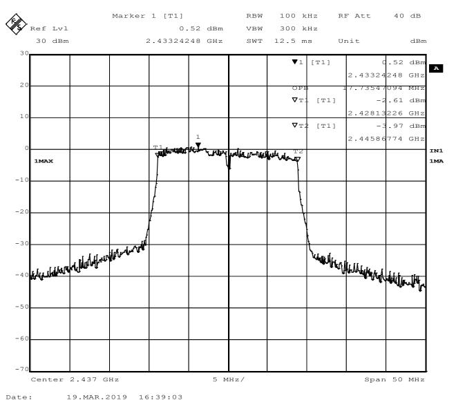
Figure 21 - 99% Occupied Bandwidth, Mid Channel, 802.11n
