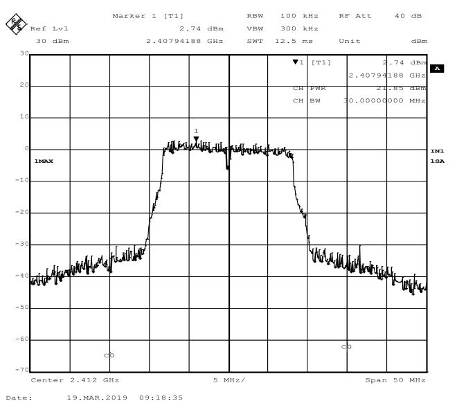
Figure 8 - Highest Measured Peak Output Power, 802.11g
