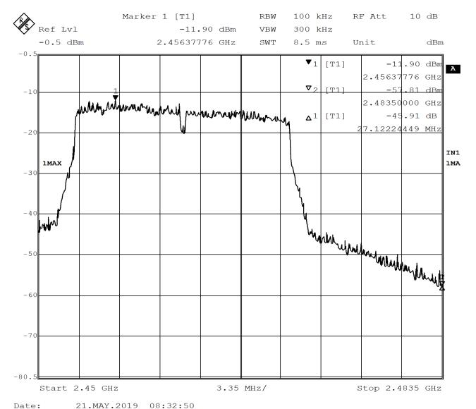
Figure 53 - Band-edge Measurement, High Channel, Fundamental, Peak
