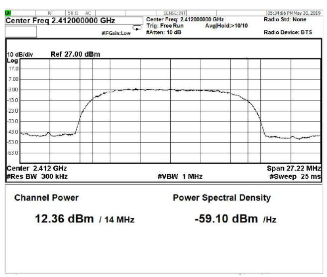
Figure 10 - Highest Measured Average Output Power, 802.11b
