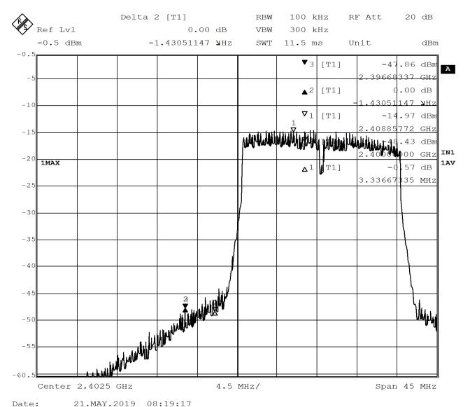
Figure 51 - Band-edge Measurement, Low Channel, Fundamental, Average
