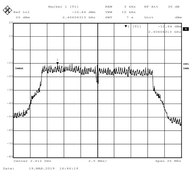
Figure 59 - Power Spectral Density, Low Channel, 802.11g
