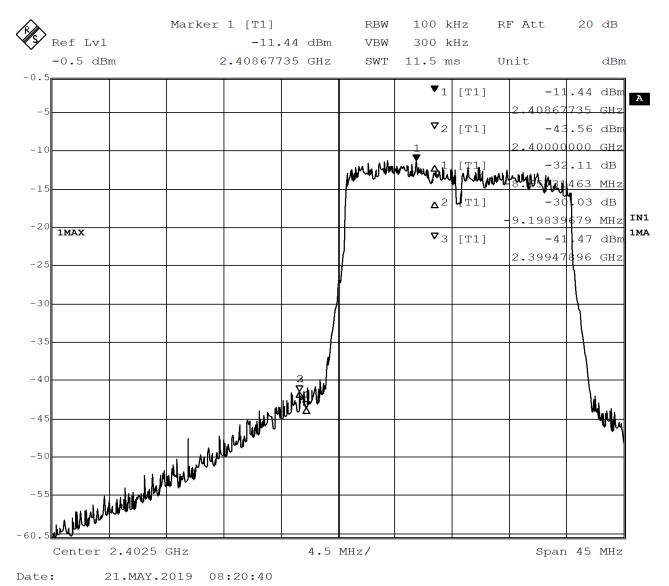
Figure 49 - Band-edge Measurement, Low Channel, Fundamental, Peak
