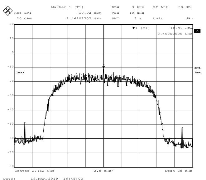
Figure 58 - Power Spectral Density, High Channel, 802.11b
