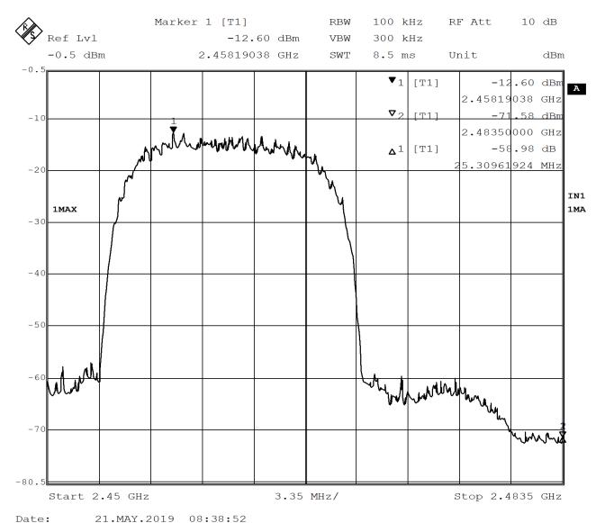
Figure 37 - Band-edge Measurement, High Channel, Fundamental, Peak
