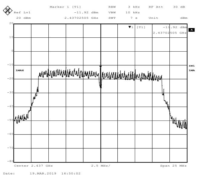
Figure 63 - Power Spectral Density, Mid Channel, 802.11n
