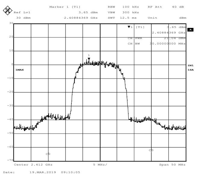
Figure 7 – Highest Measured Peak Output Power, 802.11b
