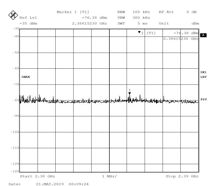
Figure 34 - Band-edge Measurement, Low Channel, Restricted Frequency, Average
