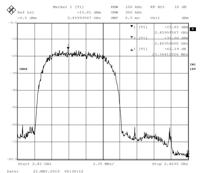
Figure 39 - Band-edge Measurement, High Channel, Fundamental, Average
