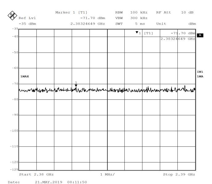
Figure 48 - Band-edge Measurement, Low Channel, Restricted Frequency, Peak
