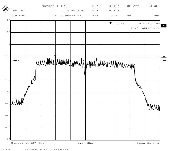
Figure 60 - Power Spectral Density, Mid Channel, 802.11g
