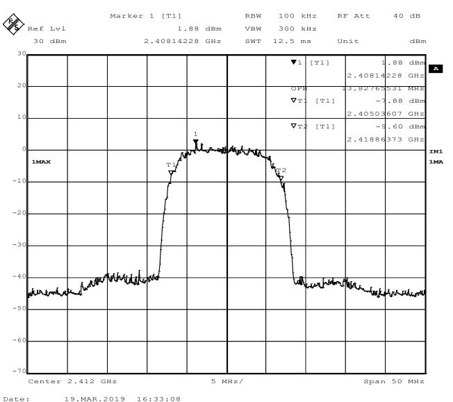
Figure 14 - 99% Occupied Bandwidth, Low Channel, 802.11b
