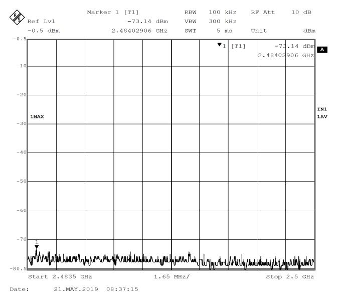
Figure 38 - Band-edge Measurement, High Channel, Restricted Frequency, Average
