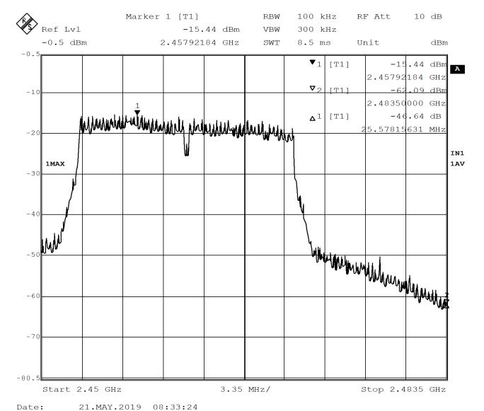
Figure 55 - Band-edge Measurement, High Channel, Fundamental, Average
