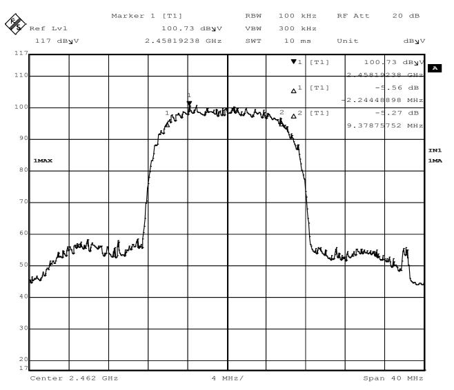
Figure 25 - 6dB Bandwidth, High Channel, 802.11b
