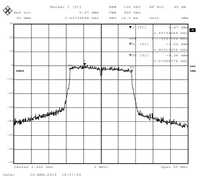
Figure 22 - 99% Occupied Bandwidth, High Channel, 802.11n
