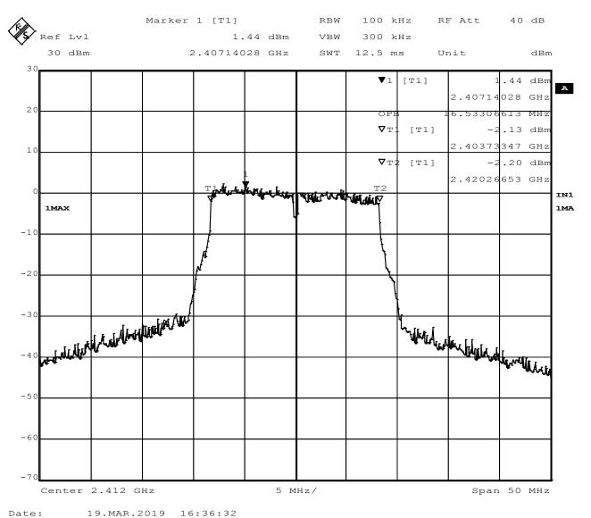
Figure 17 - 99% Occupied Bandwidth, Low Channel, 802.11g
