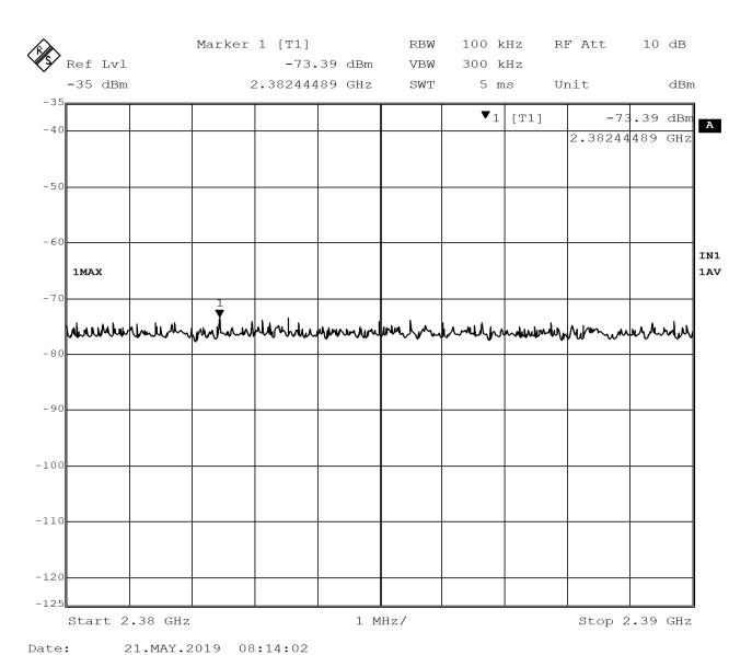
Figure 50 - Band-edge Measurement, Low Channel, Restricted Frequency, Average
