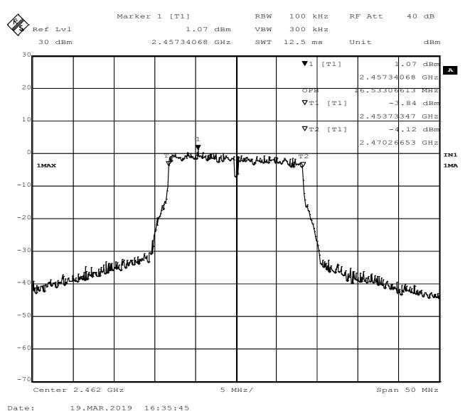
Figure 19 - 99% Occupied Bandwidth, High Channel, 802.11g
