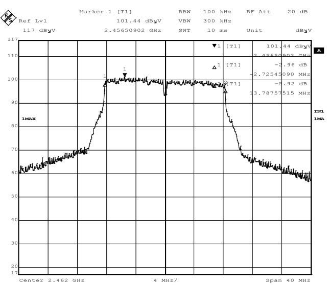
Figure 28 - 6dB Bandwidth, High Channel, 802.11g
