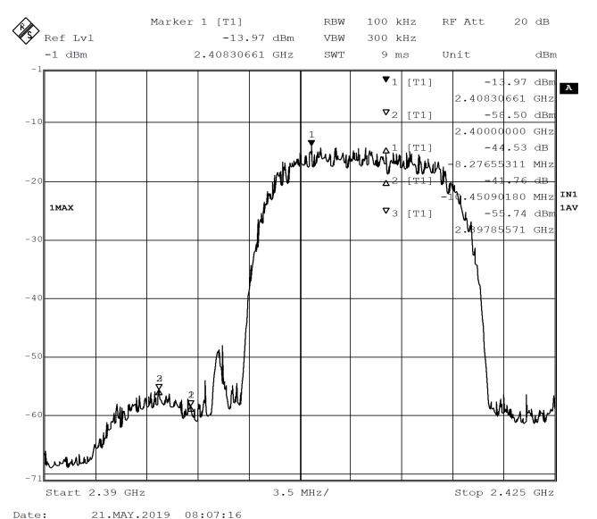
Figure 35 - Band-edge Measurement, Low Channel, Fundamental, Average
