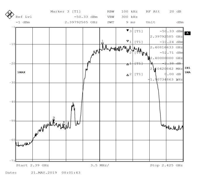
Figure 33 - Band-edge Measurement, Low Channel, Fundamental, Peak
