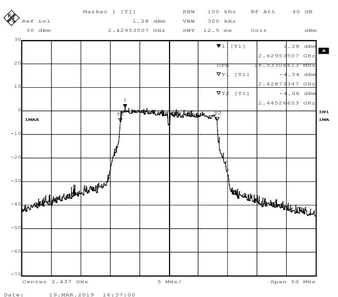
Figure 18 - 99% Occupied Bandwidth, Mid Channel, 802.11g
