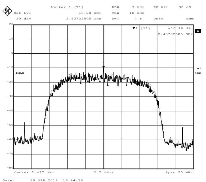
Figure 57 - Power Spectral Density, Mid Channel, 802.11b
