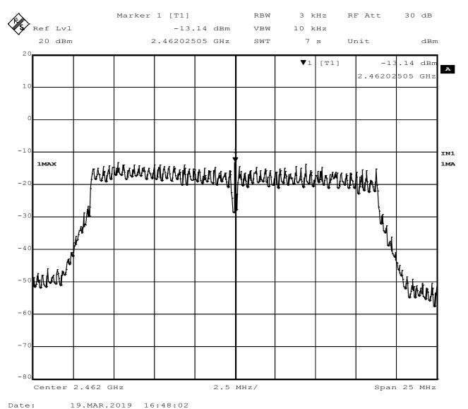
Figure 64 - Power Spectral Density, High Channel, 802.11n
