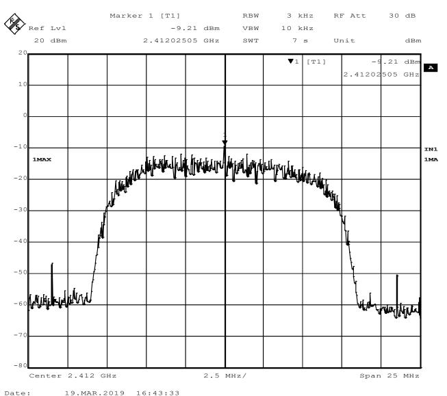
Figure 56 - Power Spectral Density, Low Channel, 802.11b
