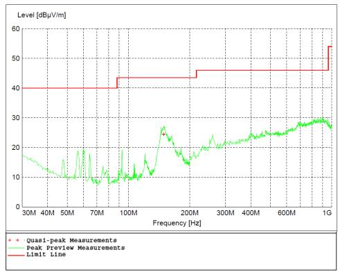
Figure 2 - Radiated Emissions Peak Plot, 30 MHz-1 GHz
